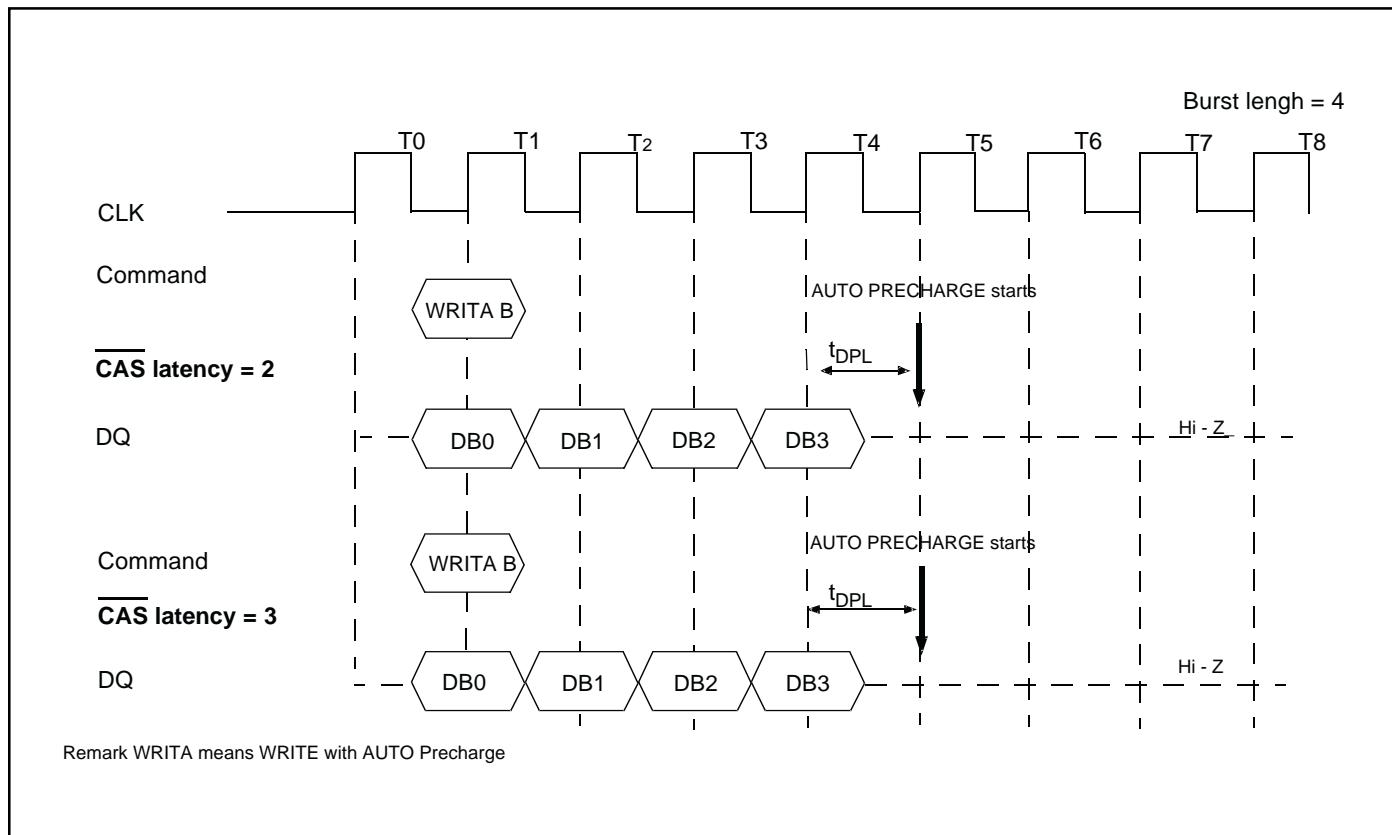
In summary, the auto precharge cycle begins relative to a reference clock that indicates the last data word is valid. In the table below, minus means clocks before the reference; plus means clocks after the reference.
