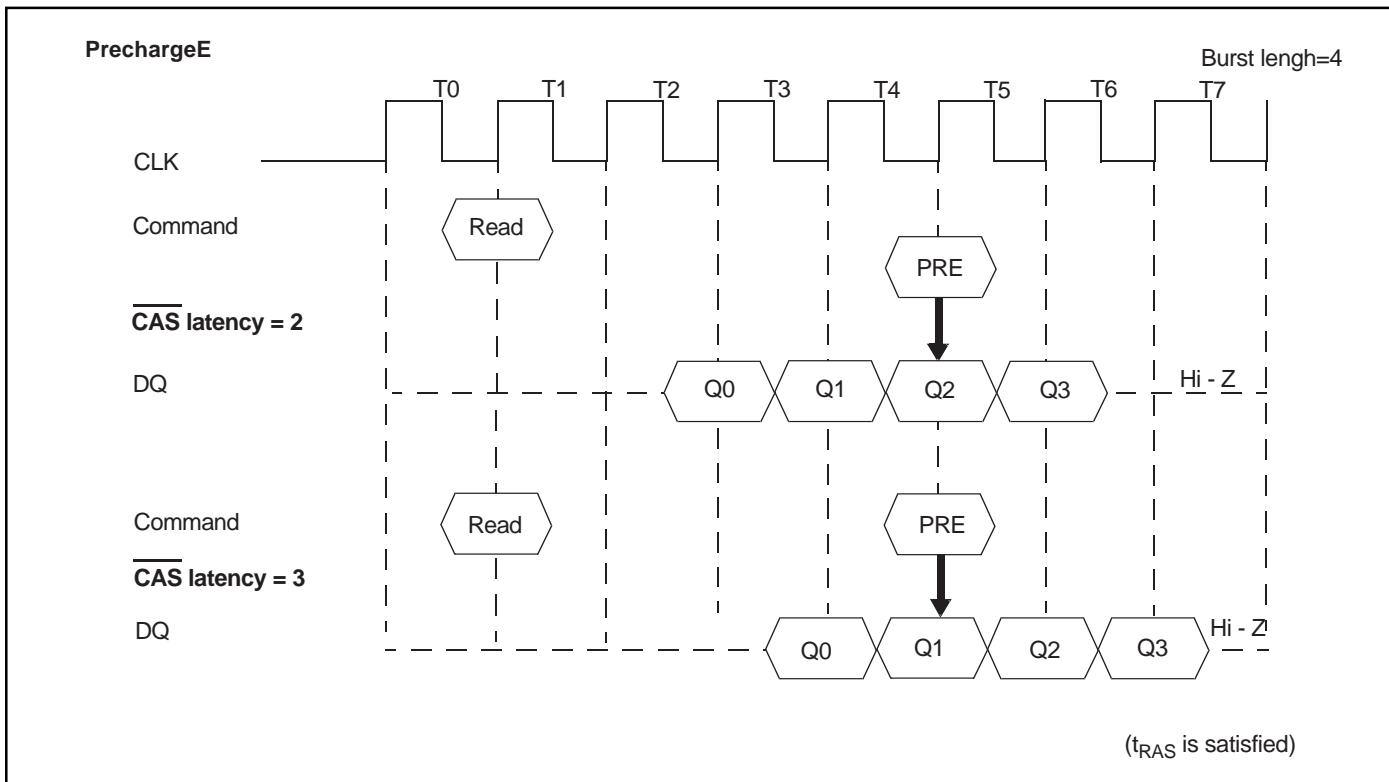
In order to write all data to the memory cell correctly, the asynchronous parameter  $t_{DPL}$  must be satisfied. The  $t_{DPL}(\text{min.})$  specification defines the earliest time that a precharge command can be asserted. The minimum number of clocks can be calculated by dividing  $t_{DPL}(\text{min.})$  with the clock cycle time.
