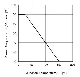
Fig.1 Power Dissipation Derating Curve
