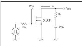
Fig.2-1 Gate Charge Measurement Circuit
