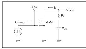
Fig.3-1 Avalanche Measurement Circuit
