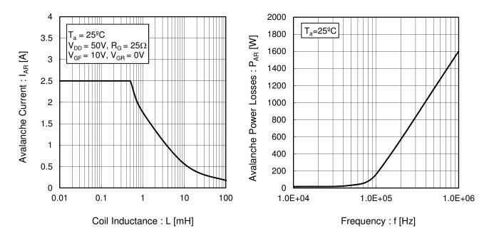
Fig.4 Avalanche Current vs Inductive Load
