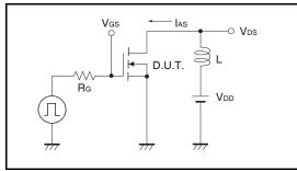
Fig.4-1 dv/dt Measurement Circuit
