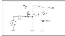
Fig.5-1 di/dt Measurement Circuit
