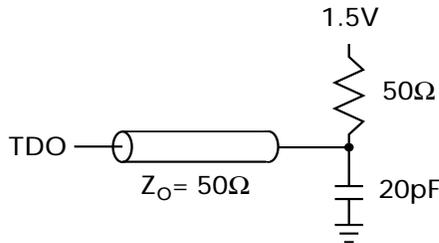
**2.5V TAP AC Output Load Equivalent**
