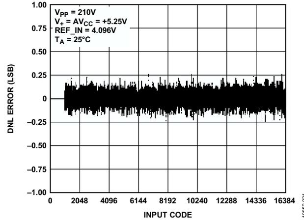
Figure 7. DNL with Full-Scale Range = 200 V
