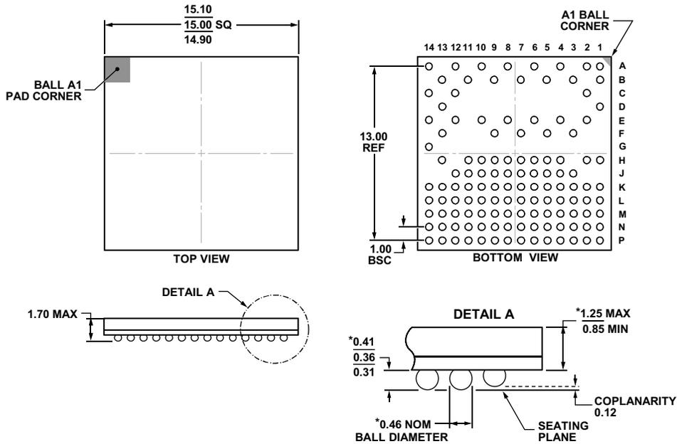
\*COMPLIANT WITH JEDEC STANDARDS MO-192-AAE-1 WITH EXCEPTION TO DIMENSIONS INDICATED BY AN ASTERISK. NOMINAL BALL SIZE IS REDUCED FROM 0.60mm TO 0.46mm.
