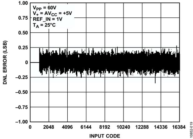
Figure 5. Differential Nonlinearity (DNL) with Full-Scale Range = 50 V
