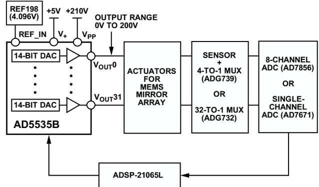
Figure 20. **AD5535B** in a MEMS-Based Optical Switch
