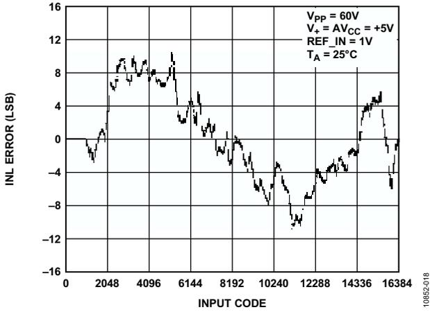
Figure 4. Integral Nonlinearity (INL) with Full-Scale Range = 50 V
