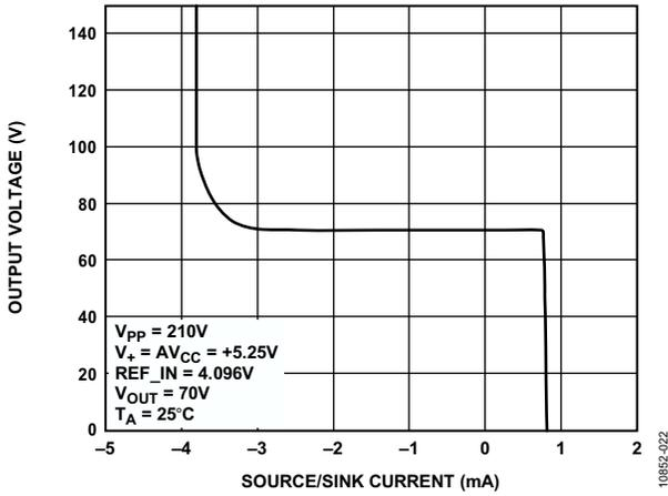
Figure 10. Output Amplifier Source and Sink Capability
