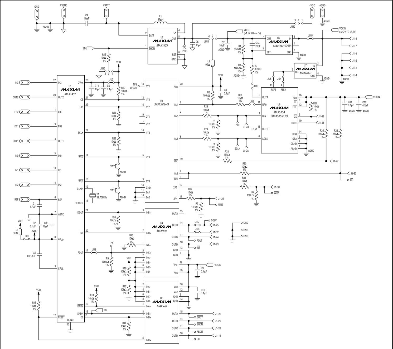
Figure 10. MAX1407 EV Kit Schematic
