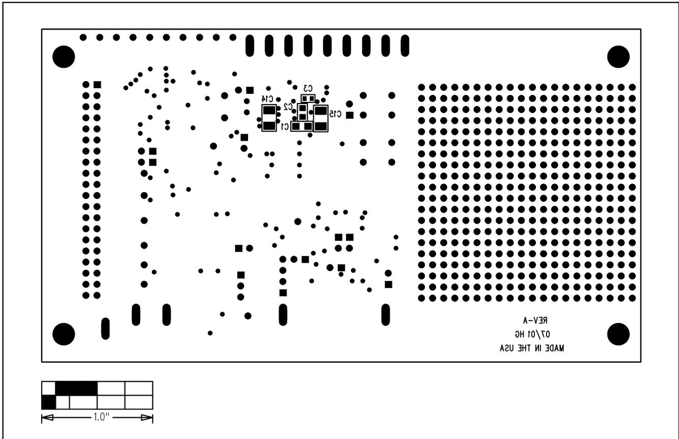
Figure 12. MAX1407 EV Kit Component Placement Guide—Solder Side
