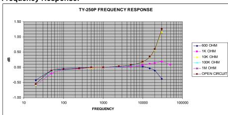
\* 600:600Ω, 10K:10KΩ, 100K:100KΩ, 1M:1MΩ, and other impedances (secondaries can all be used at  $\frac{1}{4}$  value when placed in parallel) are optional as long as input voltage is ≤4.2Vrms and current is ≤7mA.
