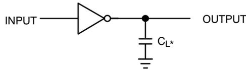
\*Includes all probe and jig capacitance.
