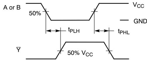
**Figure 3. Switching Waveforms**
