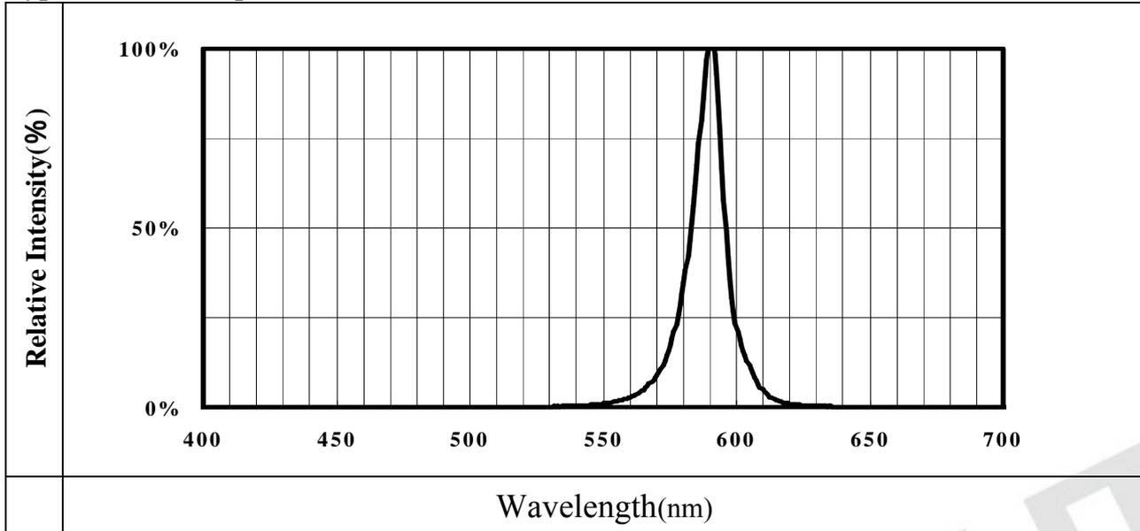
Note:  $V(\lambda)$ =Standard eye response curve;  $I_F = 20\text{mA}$
