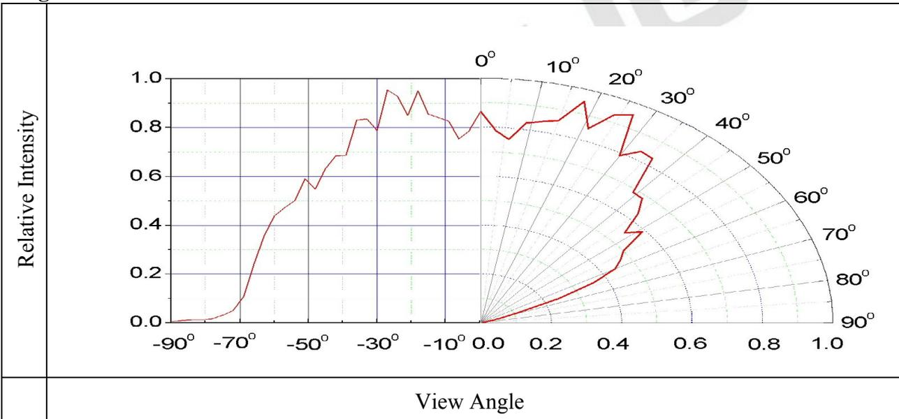
**Typical Electro-Optical Characteristics Curves**
