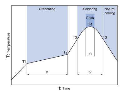
Preheating Soldering Peak Temp. Temp. Time Time Temp. Time T1 T2 T4 Т3 150°C 180°C 120s 230°C 30s 260°C 10s max.
