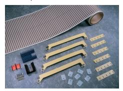
Poly-Pad® K-10 is a composite of film coated with a polyester resin. The material offers superior thermal performance for your most critical applications with a thermal resistance of 0.2°C-in²/W as well as excellent dielectric strength.
