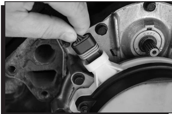
Figure 6 Disconnect the Distributor Connector.
