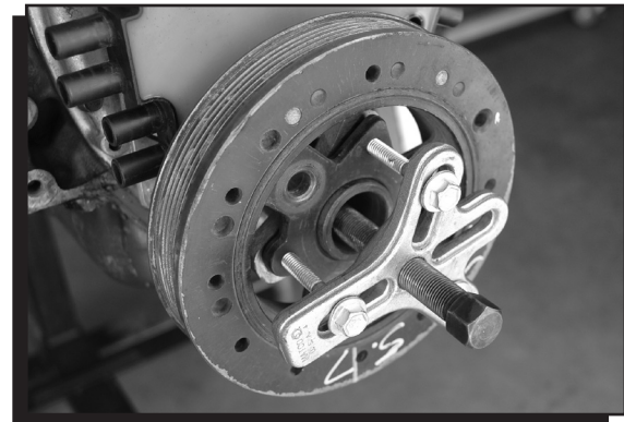
Figure 5 Removing the Hub.
