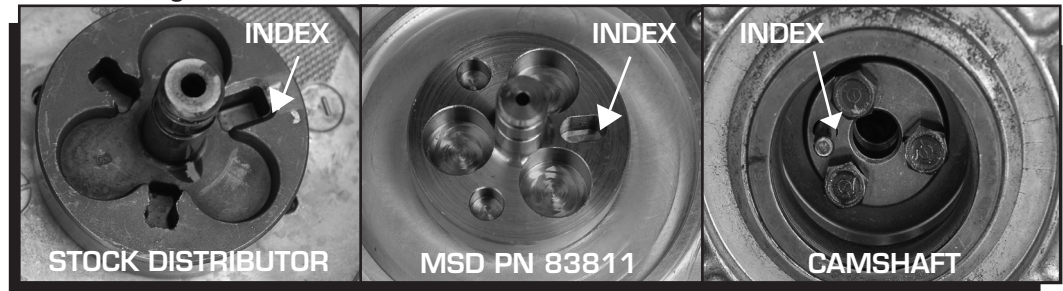
Figure 1 The Drive Mechanism of the PN 83811 Distributor.
