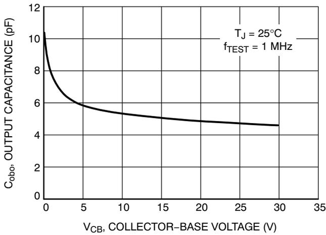
Figure 11. Output Capacitance
