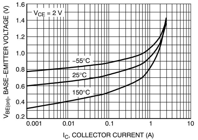
Figure 8. Base-Emitter Voltage
