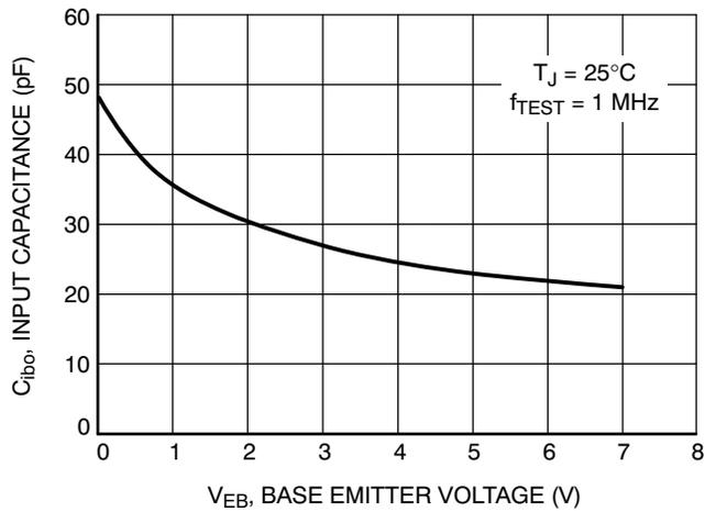
Figure 10. Input Capacitance
