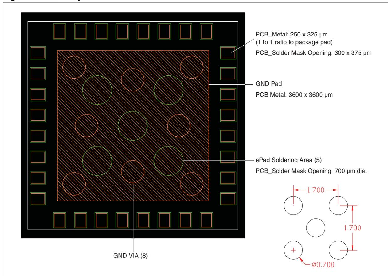
Figure 3. Stencil layout recommendation
