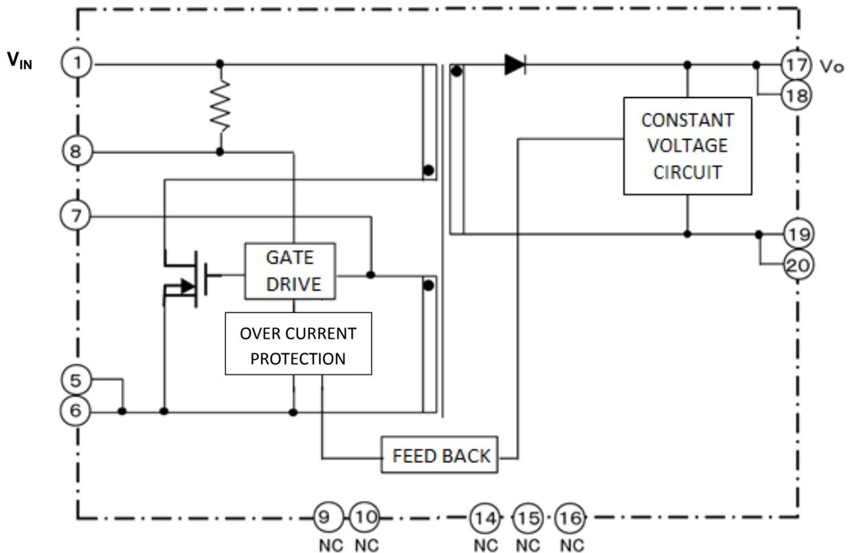
**ISOLATED TYPE DC-DC CONVERTER**
