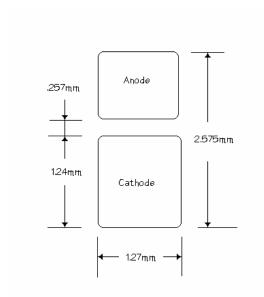
Mounting footprint, Copper (note: Silver plating will enhance Luminous Intensity)
