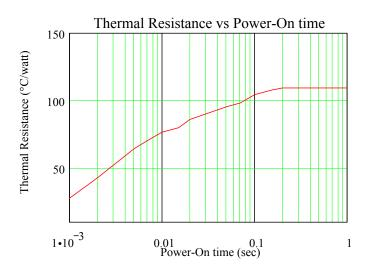
Steady State Thermal Resistance Junction-to-Optomite base metal ~ 110°C/W Thermal time constant ~ 20 mS (@ 0.632 x  $R_{\theta_{max}}$ ). Steady state temperature at ~ 500 mS.
