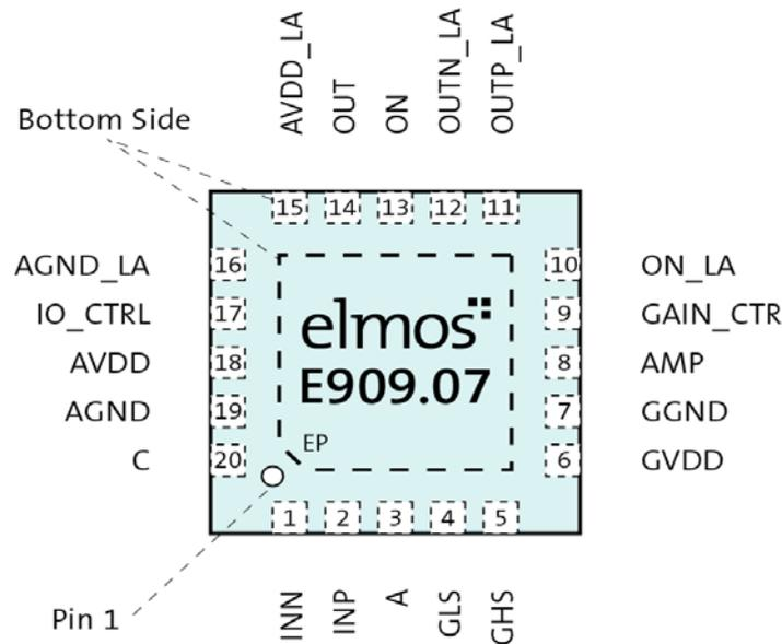
**Fig. 2: Package Pinout E909.07 (Top View)**
