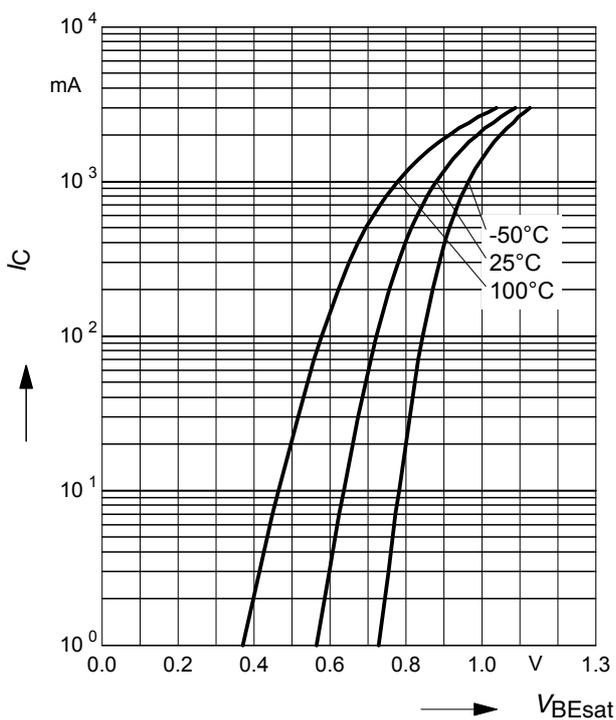
**Collector current  $I_C = f(V_{BE})$**
