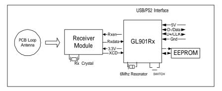
Figure 3-1: Block Diagram of RF Receiver System
