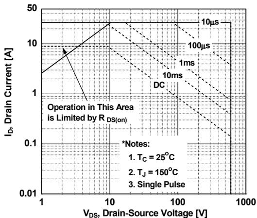
**Figure 10. Maximum Safe Operating Area \_ FCPF9N60NT**
