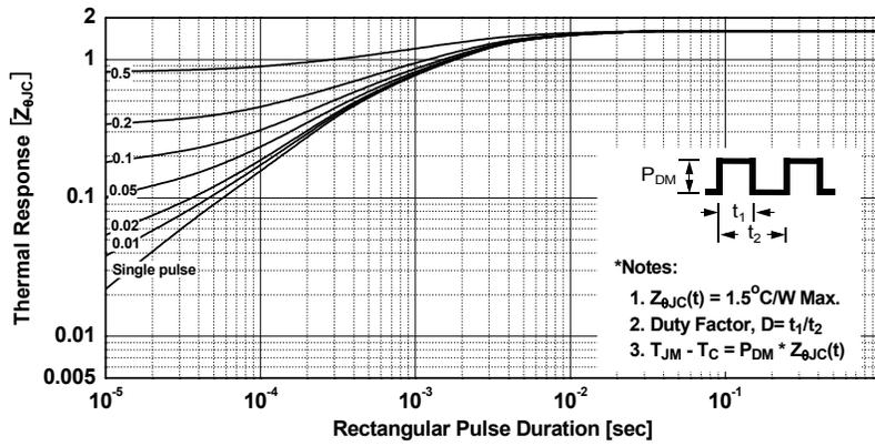
Figure 13. Transient Thermal Response Curve \_ FCPF9N60NT
