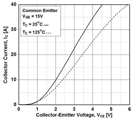
Figure 4. Transfer Characteristics
