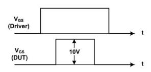
$$Qsync = \frac{1}{R_G} \cdot \int V_{R_G}(t) dt$$
