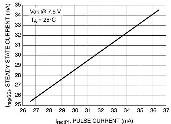
Figure 4. Steady State Current vs. Pulse Current Testing
