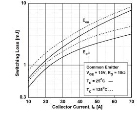
Figure 14. Turn-on Characteristics vs. Collector Current
