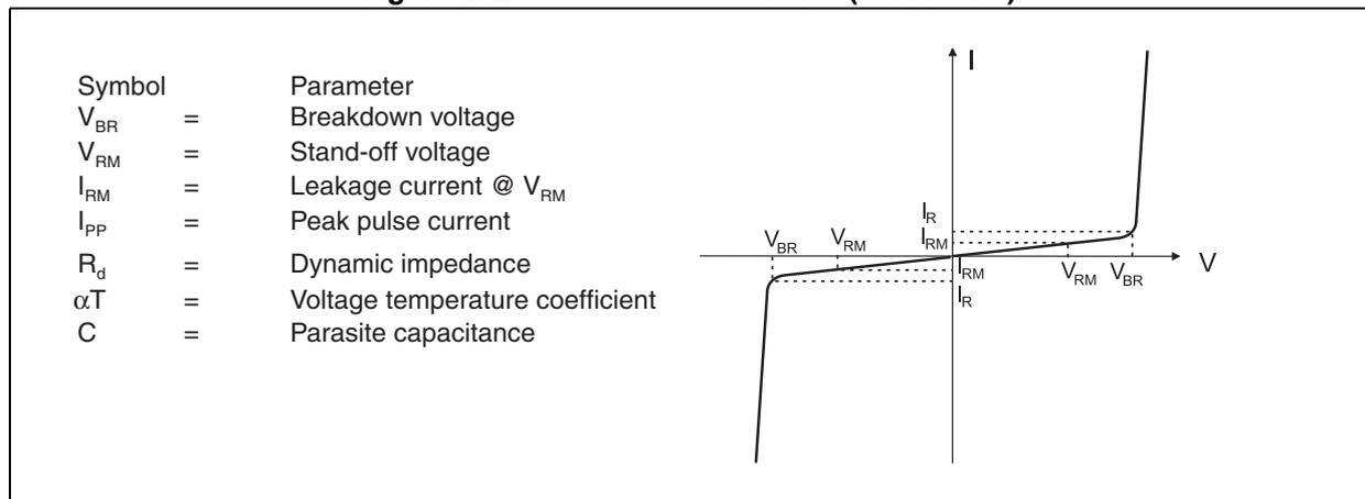
**Table 2. Electrical characteristics (values,  $T_{amb} = 25\text{ }^{\circ}\text{C}$ )**
