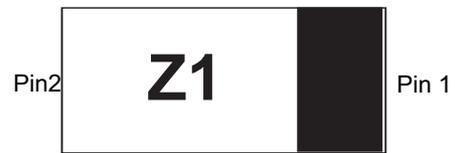
Note: Product marking may be rotated by 180° for assembly plant differentiation. In no case should this product marking be used to orient the component for its placement on a PCB. Only pin 1 mark is to be used for this purpose.
