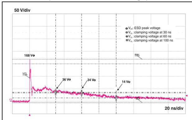
Figure 6. ESD response to IEC 61000-4-2 (-8 kV contact discharge)
