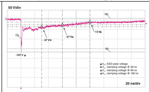
Figure 7. TLP measurements
