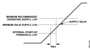
Figure 9. Start-Up Condition, Supply Slew Rate < 12.5 V/ms
