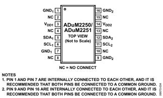
Figure 4. Pin Configuration
