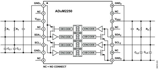
Figure 5. Timing Test Diagram
