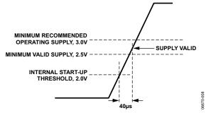
Figure 8. Start-Up Condition, Supply Slew Rate > 12.5 V/ms
