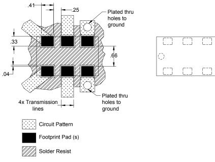
Dimensions are in Millimeters Mounting Footprint
