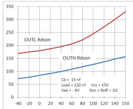
Figure 4: OUTH & OUTL Rdson's Vs Temperature ( $^\circ\text{C}$ )
