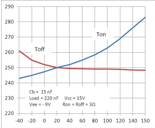
Figure 1: Ton and Toff (ns) Vs Temperature ( $^\circ\text{C}$ )
