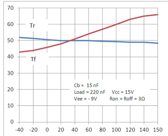
Figure 2: Tr and Tf (ns) Vs Temperature ( $^\circ\text{C}$ )
