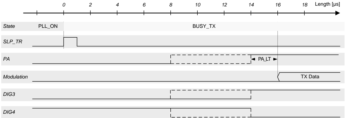
Figure 11-11. TX Power Up Ramping Control of RF Front-End for 250kb/s O-QPSK mode.
