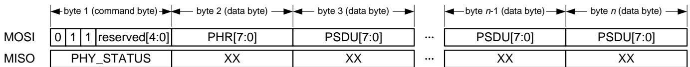
Figure 6-8. Packet Structure - Frame Write Access.
