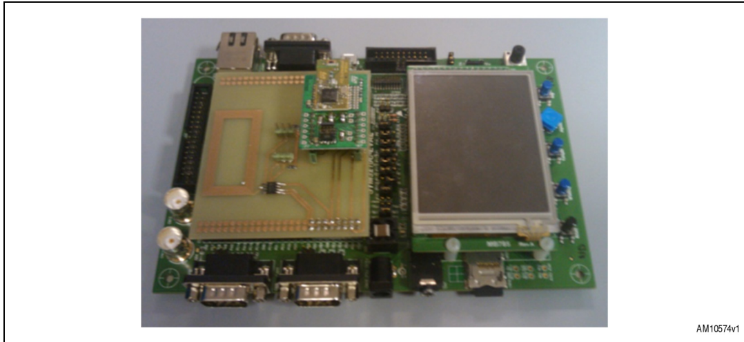
Figure 3. How to connect SPZB260-PRO adapter to the STM3210C-EVAL
