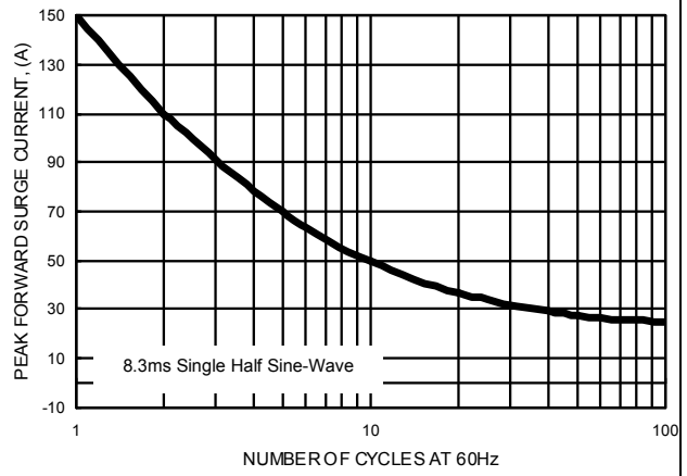
FIG.2- MAXIMUM NON-REPETITIVE SURGE CURRENT
