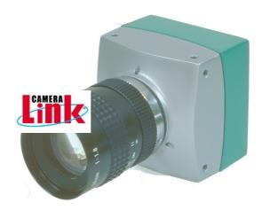
MC1302/03 can expose images synchronously or asynchronously. In synchronous (free run) mode exposure time equals frame time or, for shorter exposure times, the electronic shutter can be activated with a minimal shutter time of  $4\mu s$ . In asynchronous mode an image is exposed by an external trigger.
