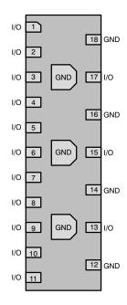
Figure 2. Pin Configuration
