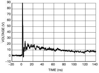
Figure 3. IEC61000-4-2 +8 kV Contact **Clamping Voltage**
