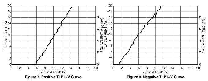
NOTE: TLP parameter:  $Z_0 = 50 \ \Omega$ ,  $t_p = 100 \ ns$ ,  $t_r = 300 \ ps$ , averaging window:  $t_1 = 30 \ ns$  to  $t_2 = 60 \ ns$ .  $V_{IEC}$  is the equivalent voltage stress level calculated at the secondary peak of the IEC 61000–4–2 waveform at  $t = 30 \ ns$  with 2 A/kV. See TLP description below for more information.
