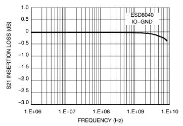
Figure 11. ESD8040 Insertion Loss
