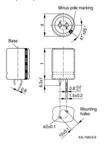
Snap-in terminals, length  $(6.3\pm1)$  mm. Also available in a shorter version with a length of (4.5-1) mm. PET insulation is marked with label "PET" on the sleeve. Safety vent on the base or on the case wall.
