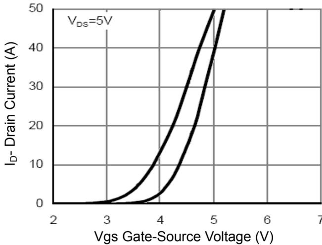
**Figure 2 Transfer Characteristics**
