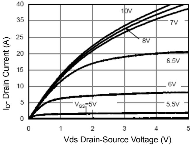
**Figure 1 Output Characteristics**
