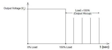
Additionally, if the  $I_{\rm O}$  is <115% but >100% for a prolong period of time (depending on the load), the Over Temperature Protection (OTP) will be activated due to high temperature on critical components. The power supply will then go into hiccup mode until the fault is removed and the mains is reapplied.
