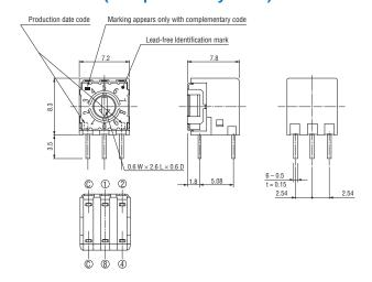
Unless otherwise specified, tolerance:  $\pm$  0.3 (Unit: mm)
