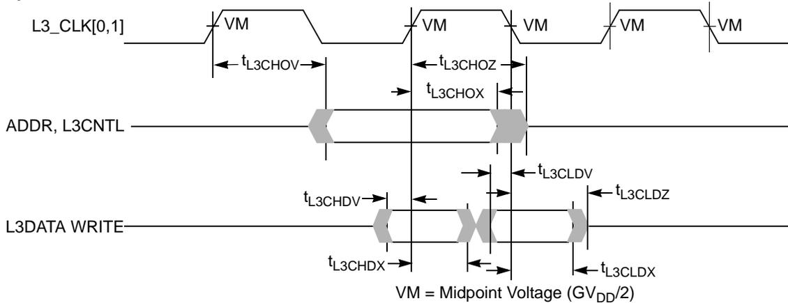
**Note:**  $t_{L3CHDV}$  and  $t_{L3CLDV}$  as drawn here will be negative numbers, that is, output valid time will be time before the clock edge.
