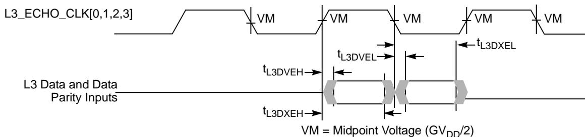
**Note:**  $t_{L3DVEH}$  and  $t_{L3DVEL}$  as drawn here will be negative numbers, that is, input setup time will be time after the clock edge.
