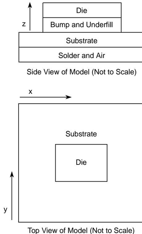
**Figure 30. Recommended Thermal Model of MPC7445 and MPC7455**
