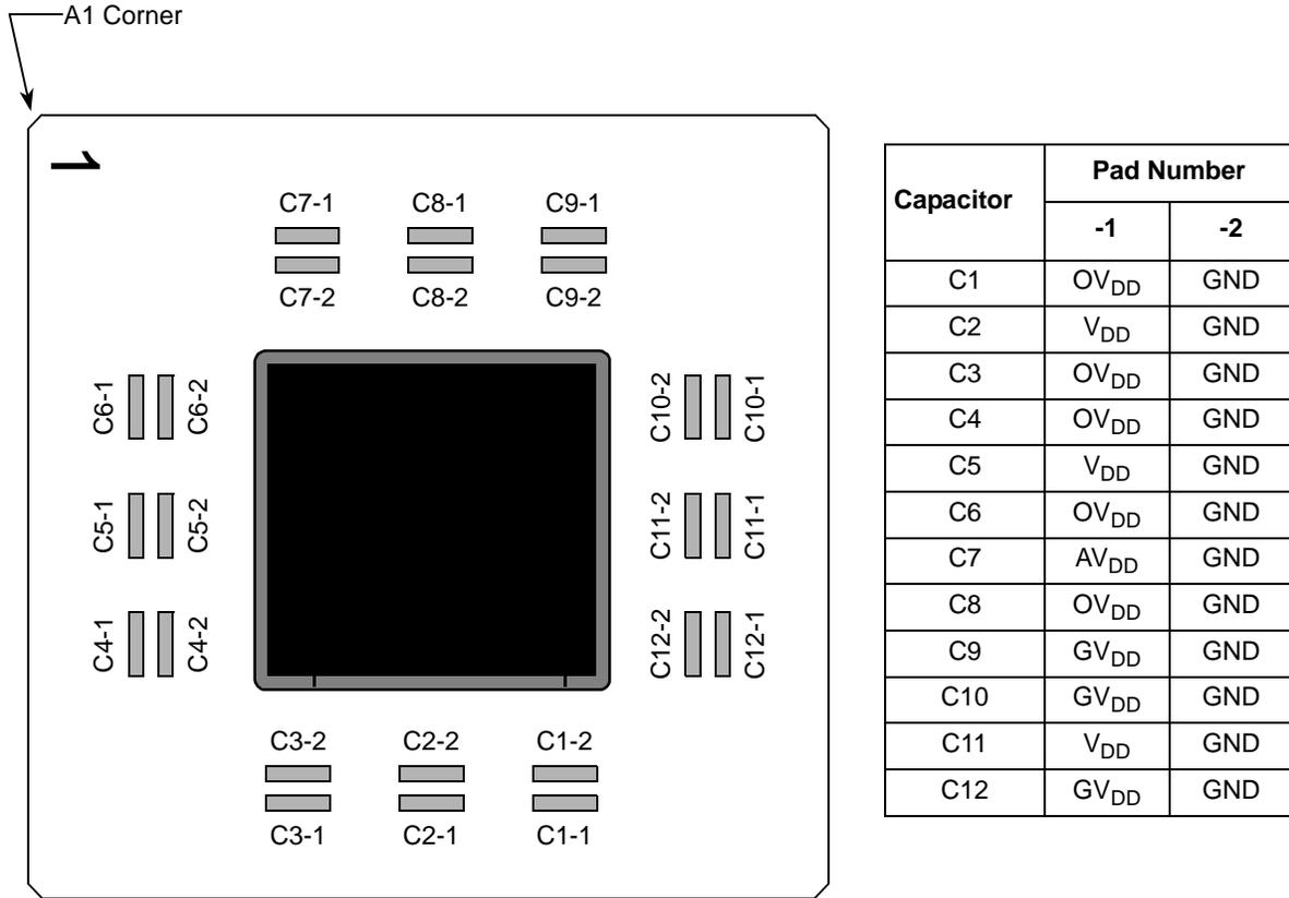
Figure 23. Substrate Bypass Capacitors for the MPC7455, 483 CBGA
