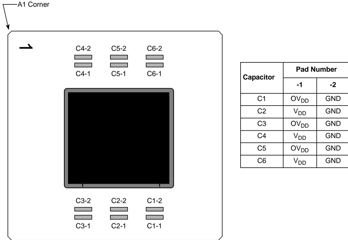
Figure 21. Substrate Bypass Capacitors for the MPC7445, 360 CBGA
