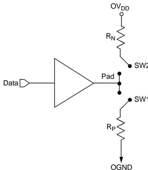
**Figure 25. Driver Impedance Measurement**
