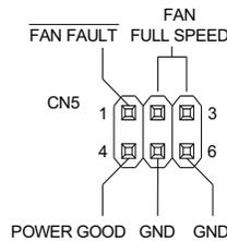
FAN FAULT: Fan Status Indication; Fan Good: Logic Level HIGH (+5V); Fan Fault: Logic Level LOW (0V)
