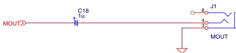
Figure 10. MOUT Output Circuit
