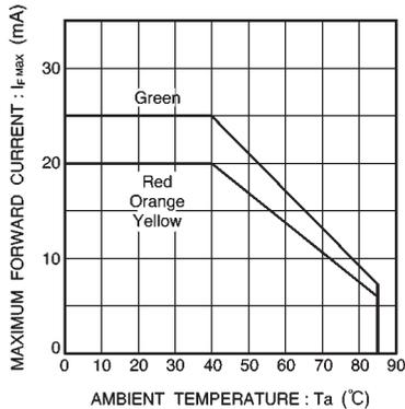
Fig. 3 Maximum forward current vs. ambient temperature
