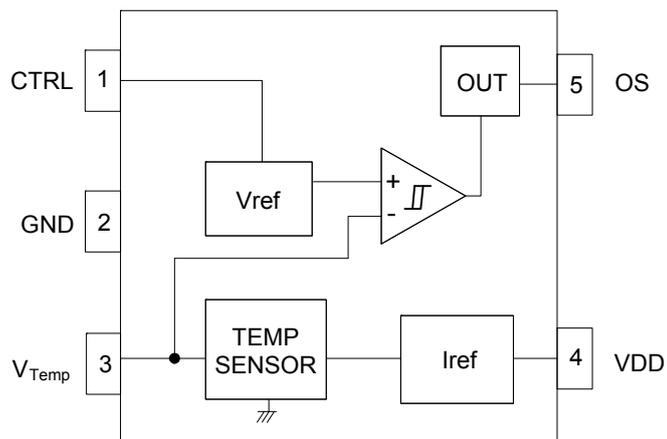
●Functional Diagram ( ex. Detection Temperature 110°C )
