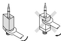
4. **Mounting direction is available in either horizontal or perpendicular.**
