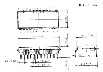
Note: Each lead pitch is 2.54mm. All leads are located within 0.25mm of their true longitudinal position with respect to No.1 and No.24 leads.
