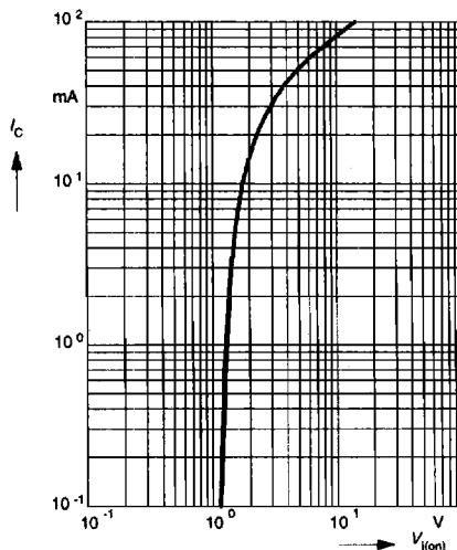
**Collector-Emitter Saturation Voltage**
