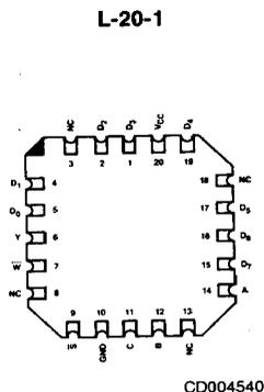
Note: Pin 1 is marked for orientation
