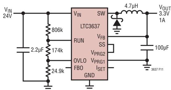
Figure 11. 24V to 3.3V, 1A Regulator at 200kHz
