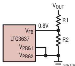
Figure 7. Setting the Output Voltage with External Resistors
