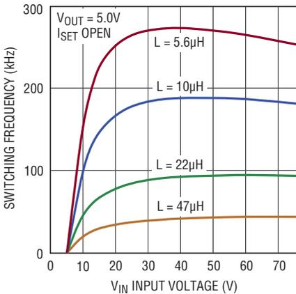
Figure 3. Switching Frequency for  $V_{OUT} = 5.0V$
