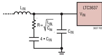
Figure 6. Series RC to Reduce  $V_{IN}$  Ringing
