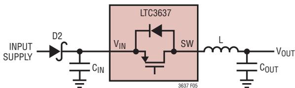
Figure 5. Preventing Current Flow to the Input
