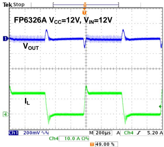
Figure 24. Transient test :1kHz, Slew rate: 2.5A/us
