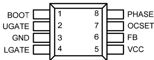
Figure 1. Pin Assignment of FP6326/A
