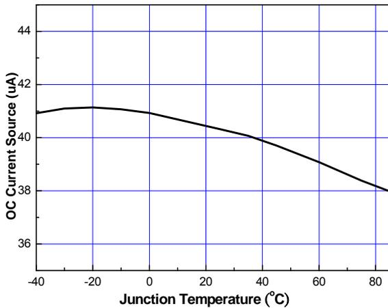
Figure 6. OC Current Source vs. Junction Temperature
