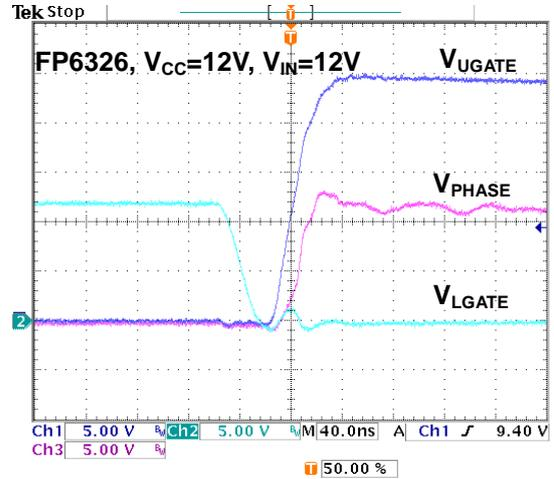
Figure 17. Switching waveform (UGATE rising)  $I_{OUT}=15A$
