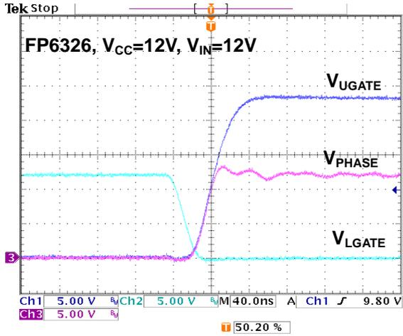
Figure 16. Switching waveform (UGATE rising)  $I_{OUT}=0A$
