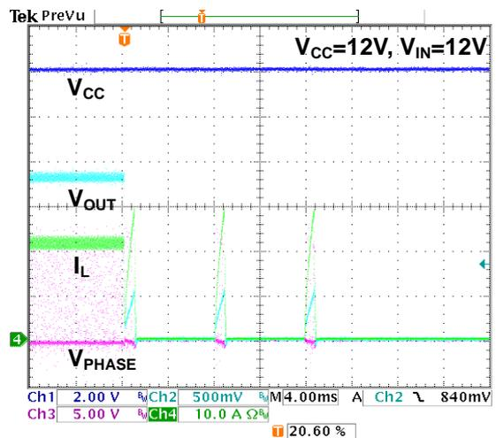
Figure 26. OCP Using DC Loading
