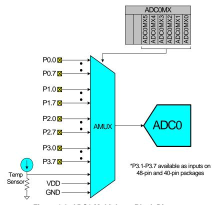
Figure 6.8. ADC0 Multiplexer Block Diagram
