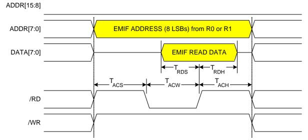
Figure 18.5. Non-multiplexed 8-bit MOVX without Bank Select Timing
