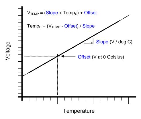
Figure 7.1. Temperature Sensor Transfer Function
