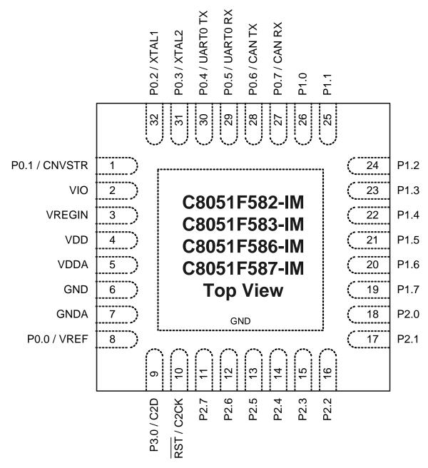
Figure 3.5. QFN-32 Pinout Diagram (Top View)
