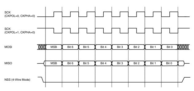
Figure 26.6. Slave Mode Data/Clock Timing (CKPHA = 0)
