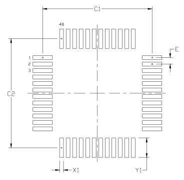
Figure 4.2. QFP-48 Landing Diagram
