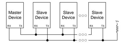
Figure 25.6. UART Multi-Processor Mode Interconnect Diagram
