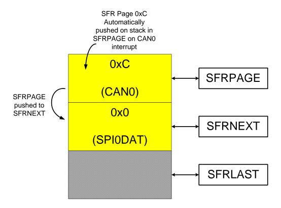
Figure 13.3. SFR Page Stack After CAN0 Interrupt Occurs
