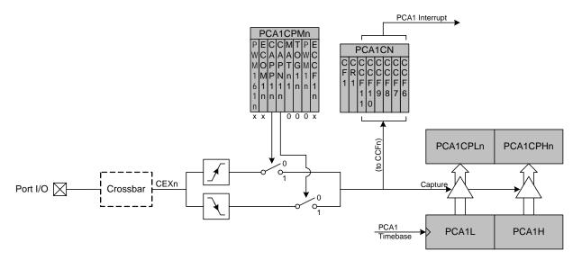
Figure 29.4. PCA1 Capture Mode Diagram
