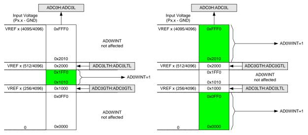
Figure 6.7. ADC Window Compare Example: Left-Justified Data
