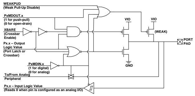
Figure 20.2. Port I/O Cell Block Diagram
