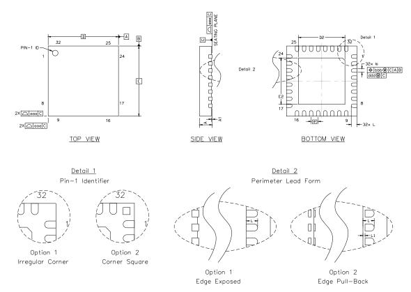
Figure 4.9. QFN-32 Package Drawing
