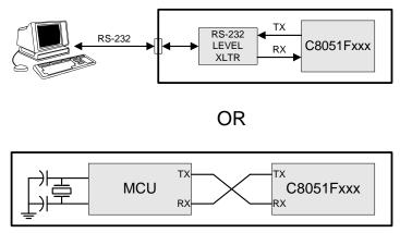
Figure 25.3. UART Interconnect Diagram
