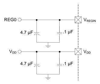
Figure 10.1. External Capacitors for Voltage Regulator Input/Output—Regulator Enabled
