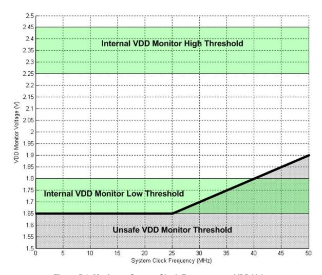
Figure 5.1. Maximum System Clock Frequency vs. VDD Voltage
