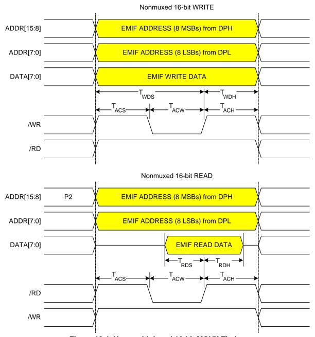
Figure 18.4. Non-multiplexed 16-bit MOVX Timing
