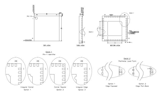
Figure 4.3. QFN-48 Package Drawing
