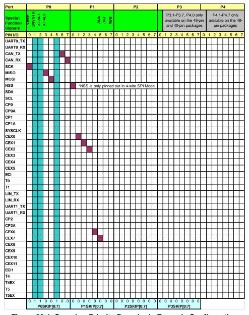
Figure 20.4. Crossbar Priority Decoder in Example Configuration
