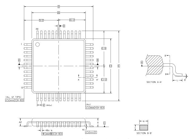
Figure 4.1. QFP-48 Package Drawing
