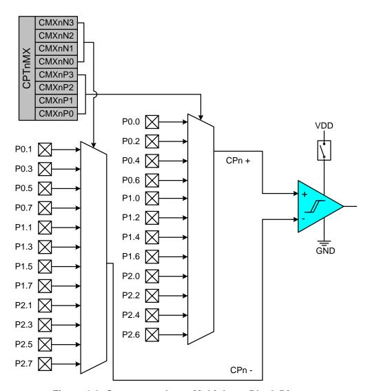
Figure 9.3. Comparator Input Multiplexer Block Diagram
