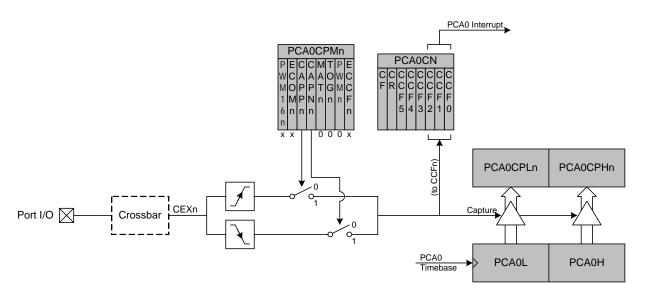
Figure 28.4. PCA0 Capture Mode Diagram
