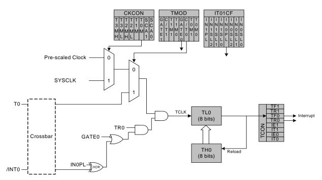
Figure 27.2. T0 Mode 2 Block Diagram
