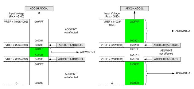
Figure 6.6. ADC Window Compare Example: Right-Justified Data
