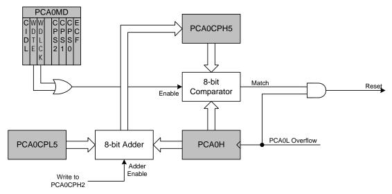
Figure 28.11. PCA0 Module 5 with Watchdog Timer Enabled
