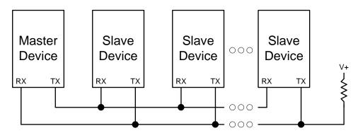
Figure 24.6. UART Multi-Processor Mode Interconnect Diagram
