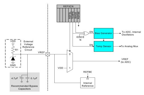
Figure 8.1. Voltage Reference Functional Block Diagram
