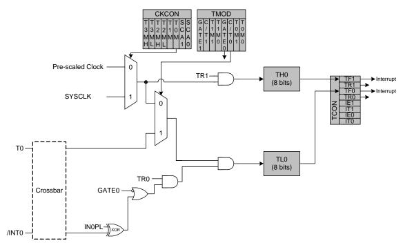
Figure 27.3. T0 Mode 3 Block Diagram
