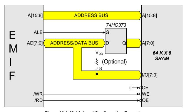
Figure 18.1. Multiplexed Configuration Example
