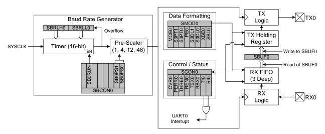
Figure 24.1. UARTO Block Diagram
