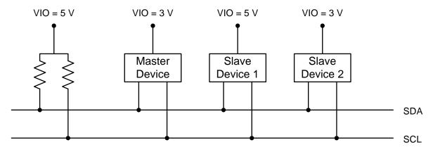
Figure 23.2. Typical SMBus Configuration
