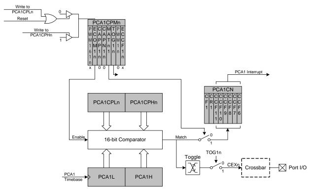
Figure 29.6. PCA1 High-Speed Output Mode Diagram
