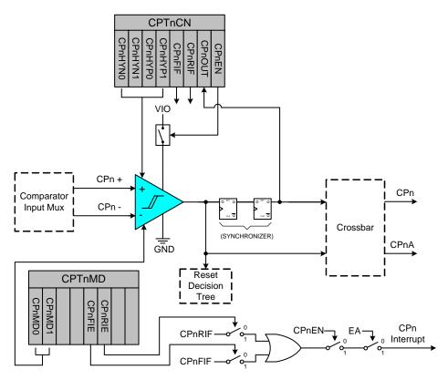
Figure 9.1. Comparator Functional Block Diagram
