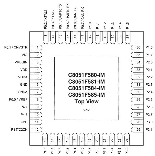
Figure 3.2. QFN-48 Pinout Diagram (Top View)
