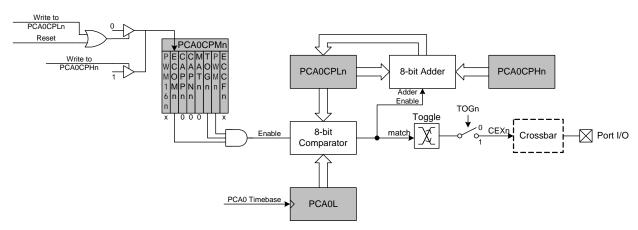
Figure 28.7. PCA0 Frequency Output Mode
