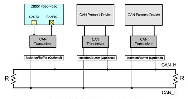
Figure 22.1. Typical CAN Bus Configuration
