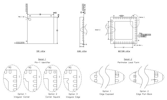
Figure 4.5. Typical QFN-40 Package Drawing
