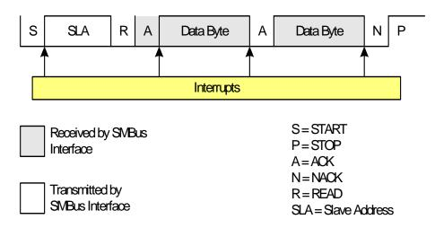
Figure 23.6. Typical Master Read Sequence
