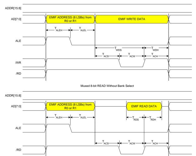
Figure 18.8. Multiplexed 8-bit MOVX without Bank Select Timing
