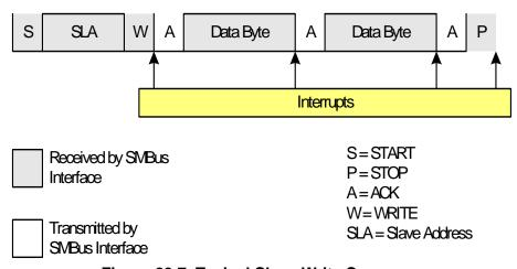
Figure 23.7. Typical Slave Write Sequence
