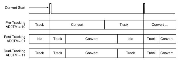
Figure 6.2. ADC0 Tracking Modes
