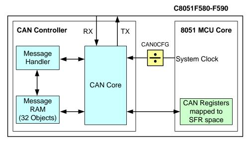
Figure 22.2. CAN Controller Diagram
