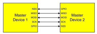
Figure 26.2. Multiple-Master Mode Connection Diagram
