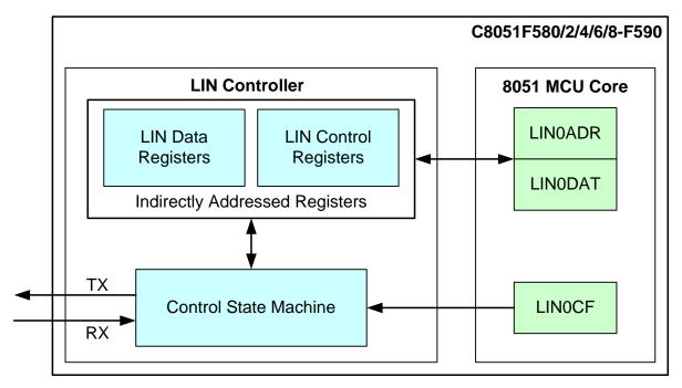
Figure 21.1. LIN Block Diagram
