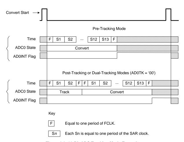
Figure 6.3. 12-Bit ADC Tracking Mode Example
