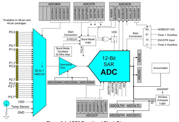
Figure 6.1. ADC0 Functional Block Diagram
