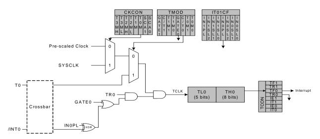
Figure 27.1. T0 Mode 0 Block Diagram
