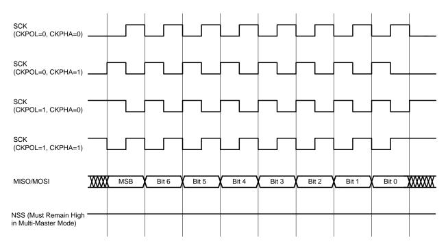
Figure 26.5. Master Mode Data/Clock Timing
