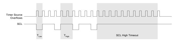
Figure 23.4. Typical SMBus SCL Generation
