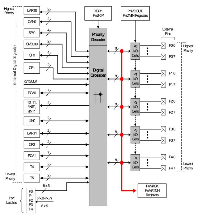
Figure 20.1. Port I/O Functional Block Diagram
