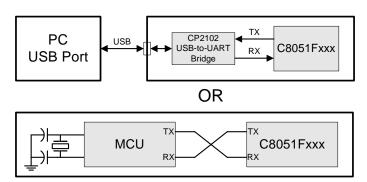
Figure 24.5. Typical UART Interconnect Diagram
