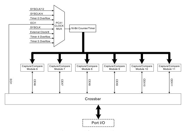
Figure 29.1. PCA1 Block Diagram
