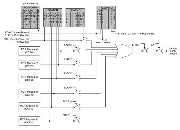
Figure 29.3. PCA1 Interrupt Block Diagram
