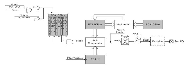
Figure 29.7. PCA1 Frequency Output Mode
