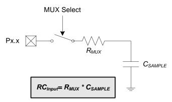
Figure 6.5. ADC0 Equivalent Input Circuit
