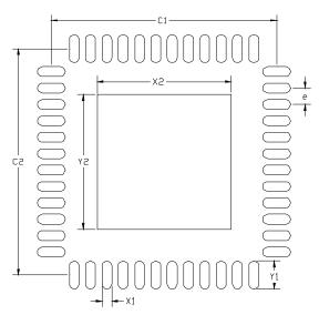
Figure 4.4. QFN-48 Landing Diagram
