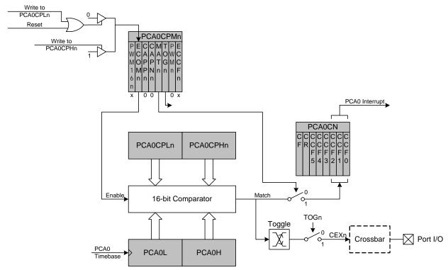
Figure 28.6. PCA0 High-Speed Output Mode Diagram
