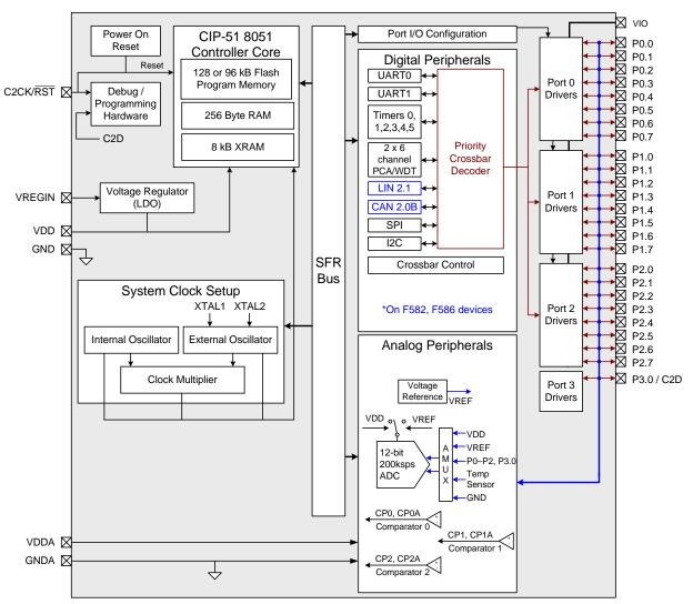
Figure 1.3. C8051F582/3/6/7 Block Diagram
