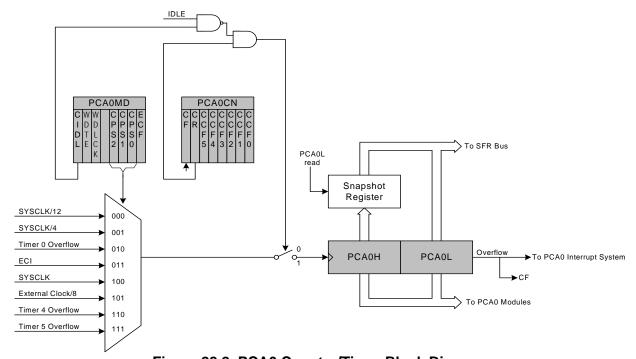
Figure 28.2. PCA0 Counter/Timer Block Diagram
