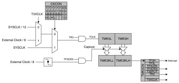
Figure 27.9. Timer 3 External Oscillator Capture Mode Block Diagram
