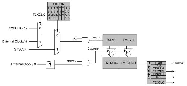
Figure 27.6. Timer 2 External Oscillator Capture Mode Block Diagram
