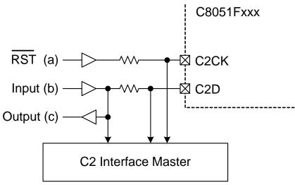
Figure 30.1. Typical C2 Pin Sharing
