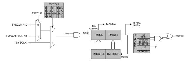
Figure 27.7. Timer 3 16-Bit Mode Block Diagram
