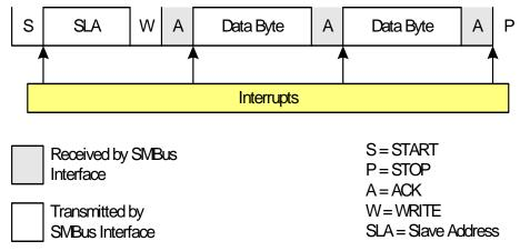
Figure 23.5. Typical Master Write Sequence
