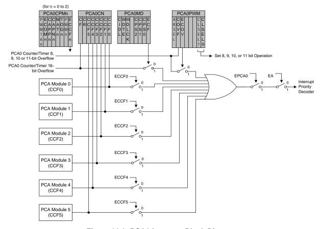
Figure 28.3. PCA0 Interrupt Block Diagram
