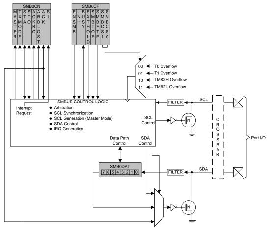
Figure 23.1. SMBus Block Diagram
