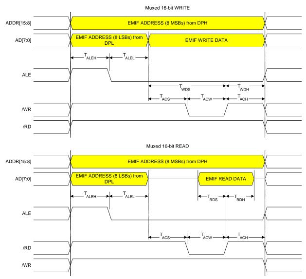
Figure 18.7. Multiplexed 16-bit MOVX Timing
