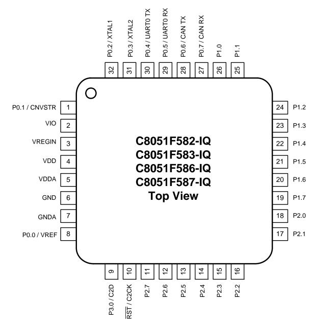
Figure 3.4. QFP-32 Pinout Diagram (Top View)
