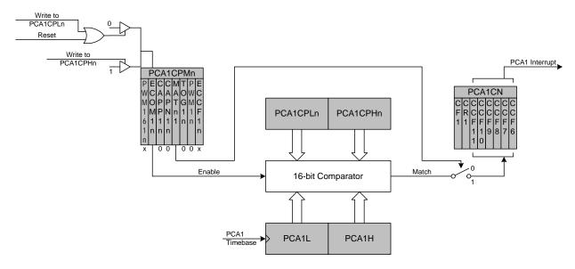
Figure 29.5. PCA1 Software Timer Mode Diagram
