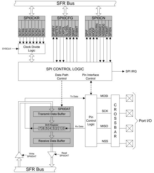
Figure 26.1. SPI Block Diagram
