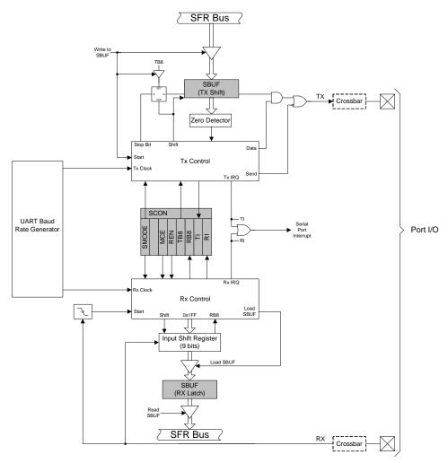
Figure 25.1. UART1 Block Diagram
