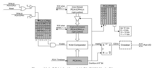
Figure 29.9. PCA1 9, 10 and 11-Bit PWM Mode Diagram
