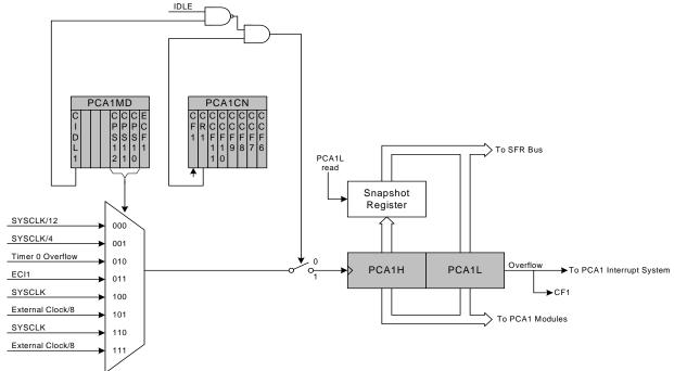
Figure 29.2. PCA1 Counter/Timer Block Diagram
