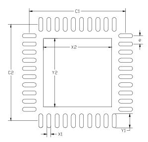
Figure 4.6. QFN-40 Landing Diagram
