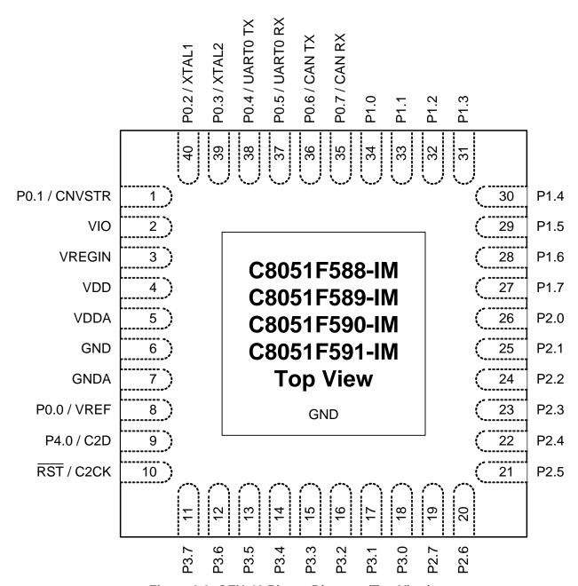
Figure 3.3. QFN-40 Pinout Diagram (Top View)
