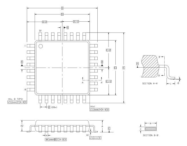
Figure 4.7. QFP-32 Package Drawing
