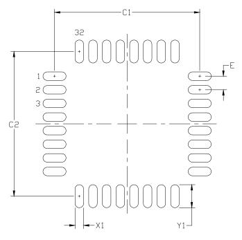
Figure 4.8. QFP-32 Package Drawing
