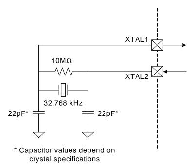
Figure 19.3. External 32.768 kHz Quartz Crystal Oscillator Connection Diagram
