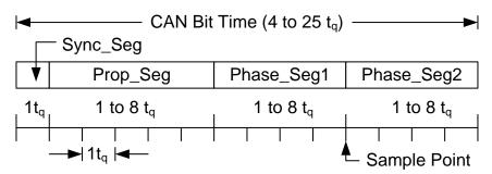
Figure 22.3. Four segments of a CAN Bit
