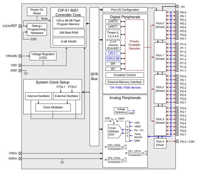
Figure 1.2. C8051F588/9-F590/1 Block Diagram
