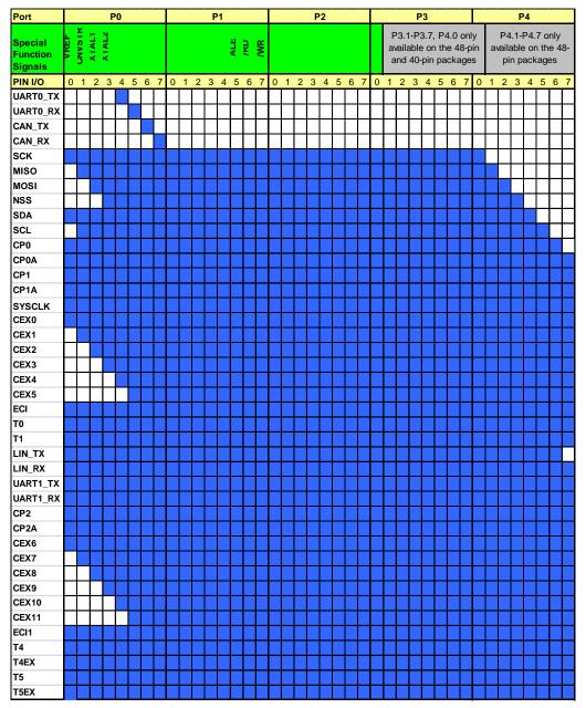
Figure 20.3. Peripheral Availability on Port I/O Pins
