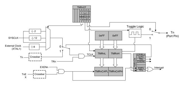
Figure 27.10. Timer 4 and 5 Capture Mode Block Diagram
