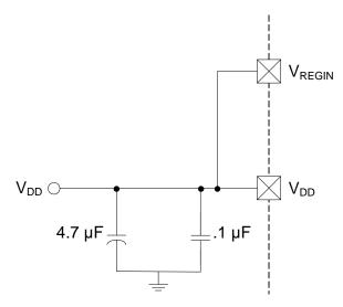
Figure 10.2. External Capacitors for Voltage Regulator Input/Output—Regulator Disabled
