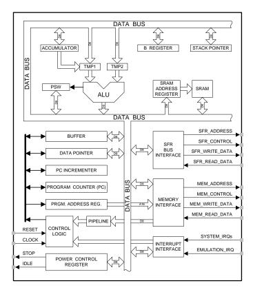
Figure 11.1. CIP-51 Block Diagram
