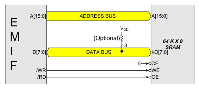
Figure 18.2. Non-multiplexed Configuration Example
