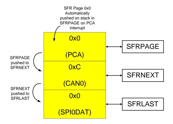
Figure 13.4. SFR Page Stack Upon PCA Interrupt Occurring During a CAN0 ISR
