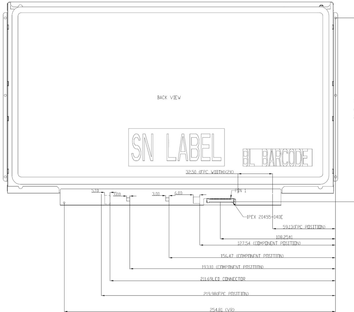
Note: Prevention IC damage, IC positions not allowed any overlap over these areas.
