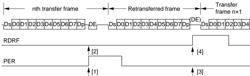
**Figure 13-11 Retransfer Operation in SCI Receive Mode**
