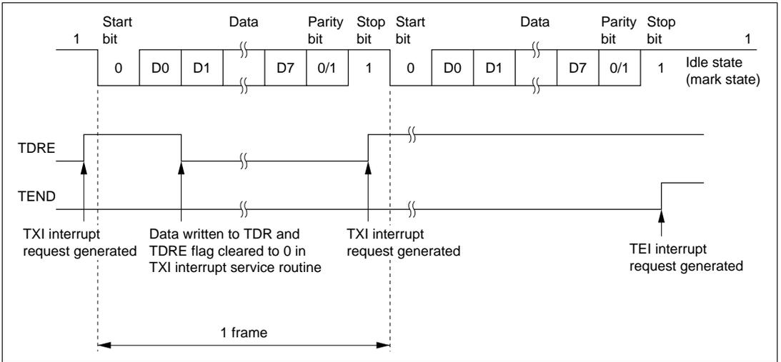
**Figure 12-6 Example of Operation in Transmission in Asynchronous Mode
