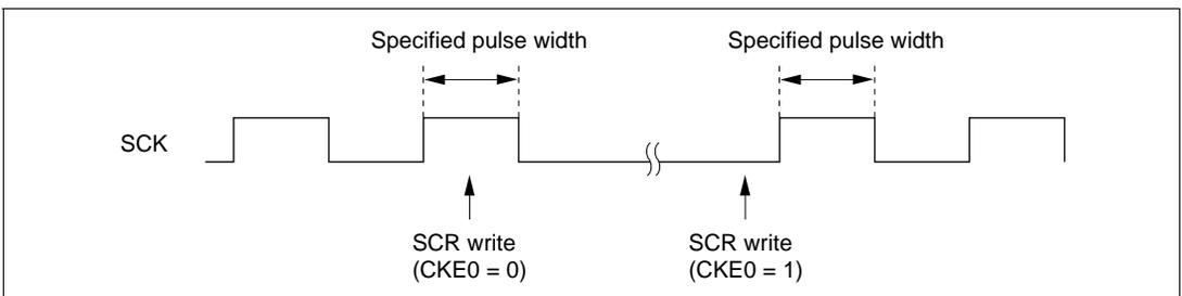
**Figure 13-8 Timing for Fixing Clock Output Level**
