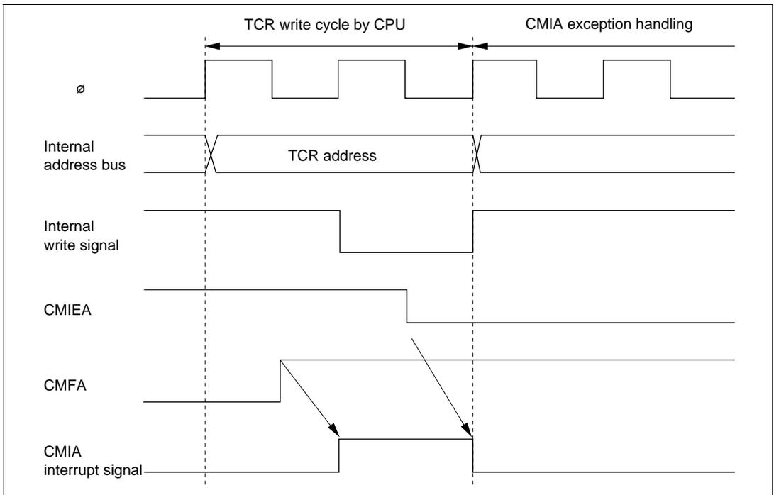
**Figure 5-9 Contention between Interrupt Generation and Disabling**
