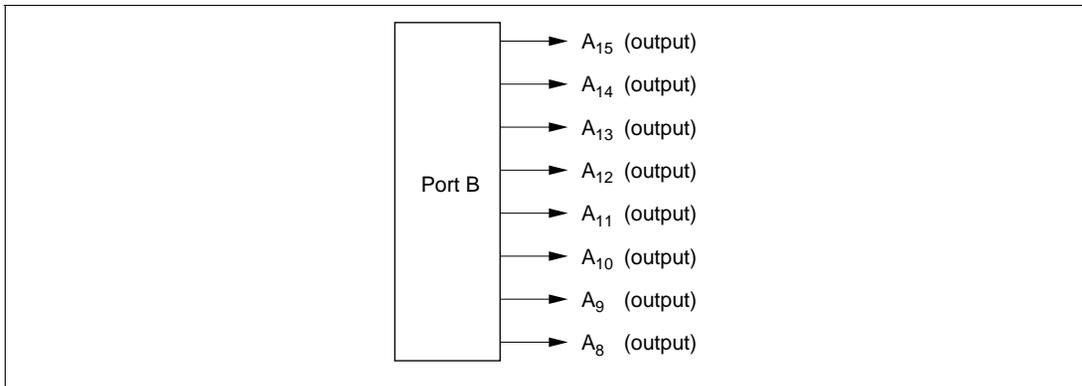
**Figure 8-11 Port B Pin Functions (Modes 1, 4, and 5)**
