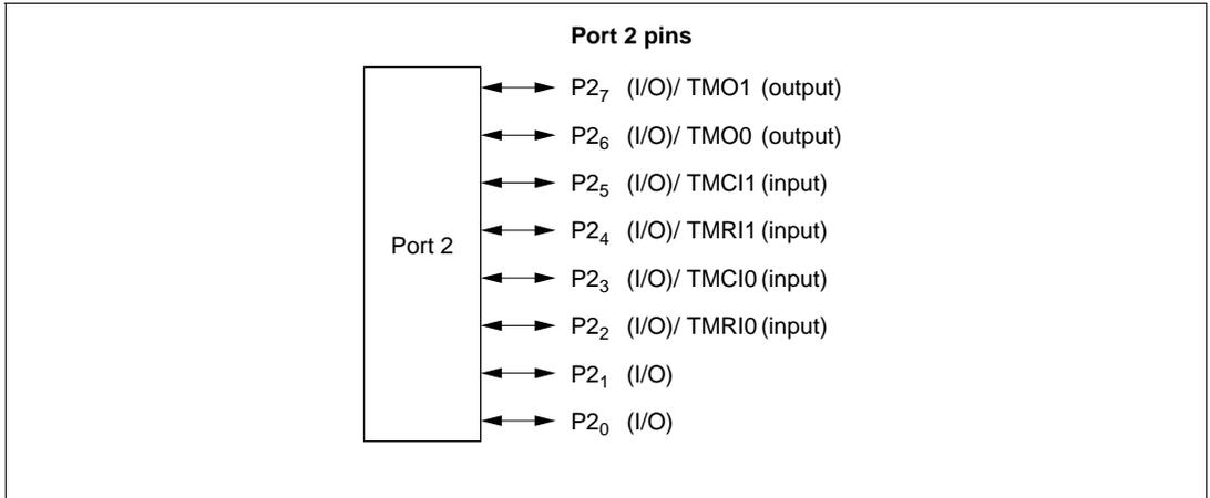
**Figure 8-2 Port 2 Pin Functions**
