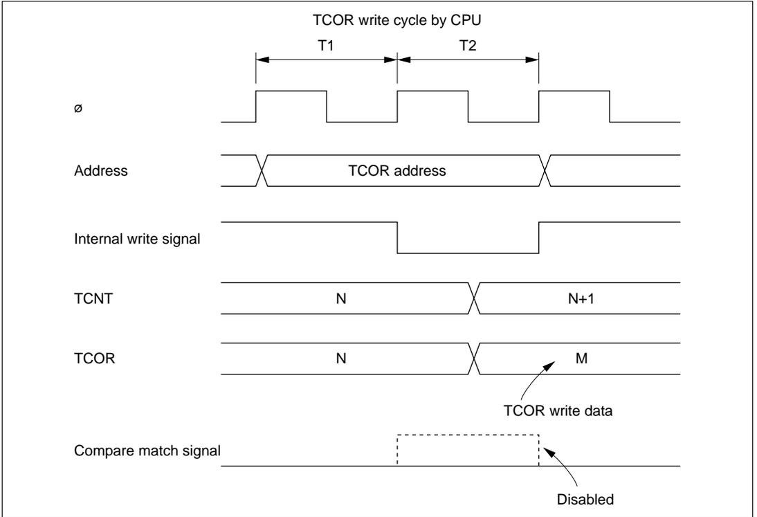
**Figure 10-12** Contention between TCOR Write and Compare Match
