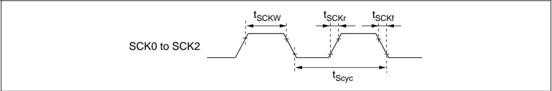
**Figure 19-22 SCK Clock Input Timing**
