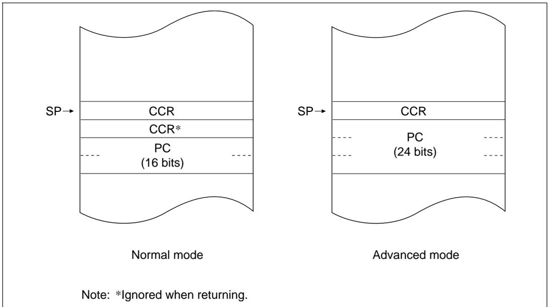
**Figure 2-16 Stack Structure after Exception Handling (Examples)**
