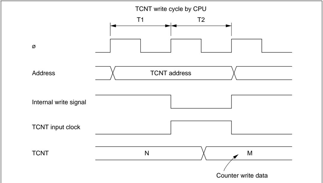
**Figure 10-11 Contention between TCNT Write and Increment**
