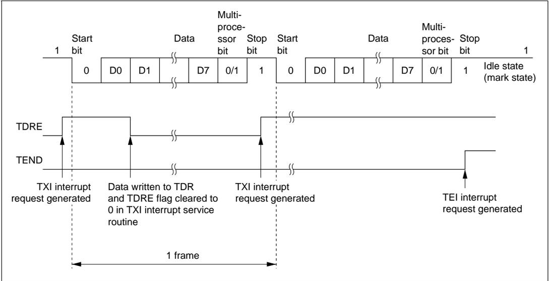
**Figure 12-11 Example of SCI Operation in Transmission
