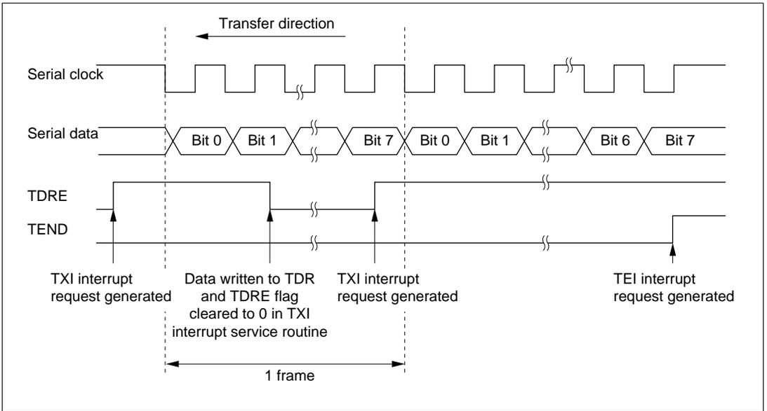
**Figure 12-17 Example of SCI Operation in Transmission**
