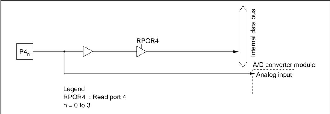
Figure C-4 Port 4 Block Diagram (Pins  $P4_0$  to  $P4_3$ )
