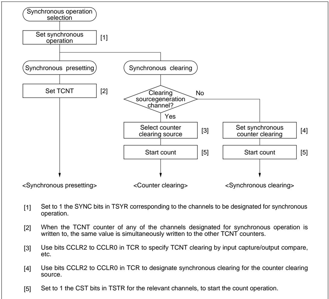
**Figure 9-14 Example of Synchronous Operation Setting Procedure**
