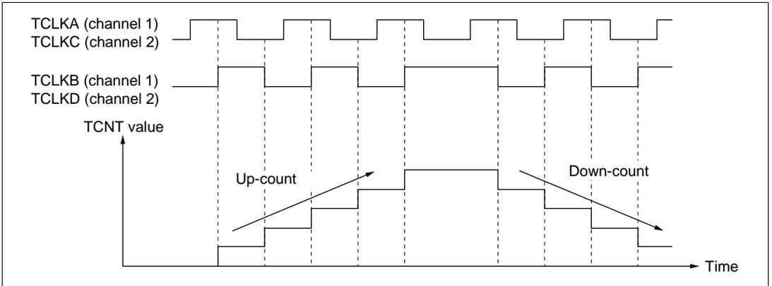
**Figure 9-29 Example of Phase Counting Mode 4 Operation**
