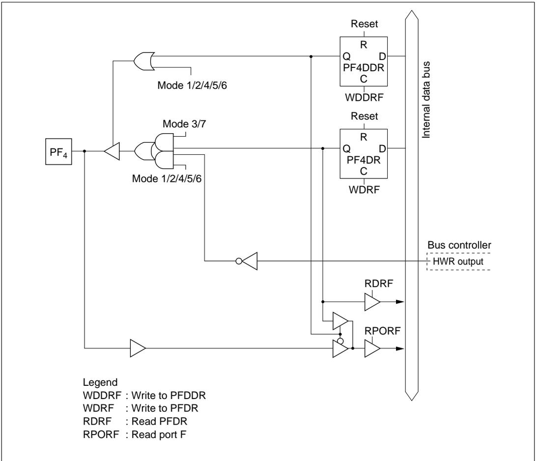
**Figure C-11 (e) Port F Block Diagram (Pin PF<sub>4</sub>)**
