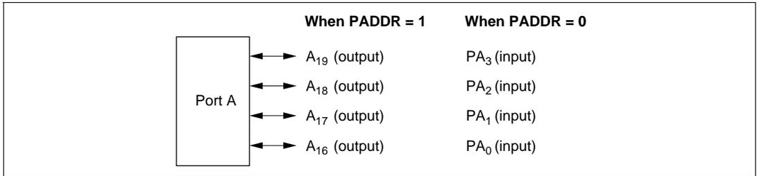
**Figure 8-9 Port A Pin Functions (Mode 6)**
