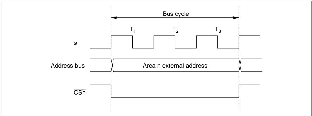
**Figure 6-3  $\overline{CSn}$  Signal Output Timing ( $n = 0$  to 3)**
