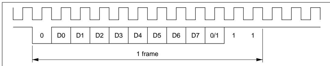
**Figure 12-3 Relation between Output Clock and Transfer Data Phase
