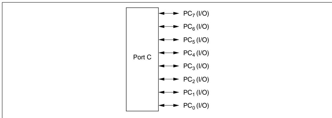
**Figure 8-17 Port C Pin Functions (Modes 3 and 7)**
