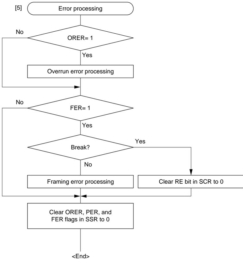
**Figure 12-12 Sample Multiprocessor Serial Reception Flowchart (cont)**
