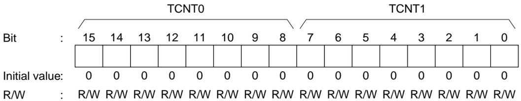
TCNT0 and TCNT1 are 8-bit readable/writable up-counters that increment on pulses generated from an internal or external clock source. This clock source is selected by clock select bits CKS2 to CKS0 of TCR. The CPU can read or write to TCNT0 and TCNT1 at all times.
