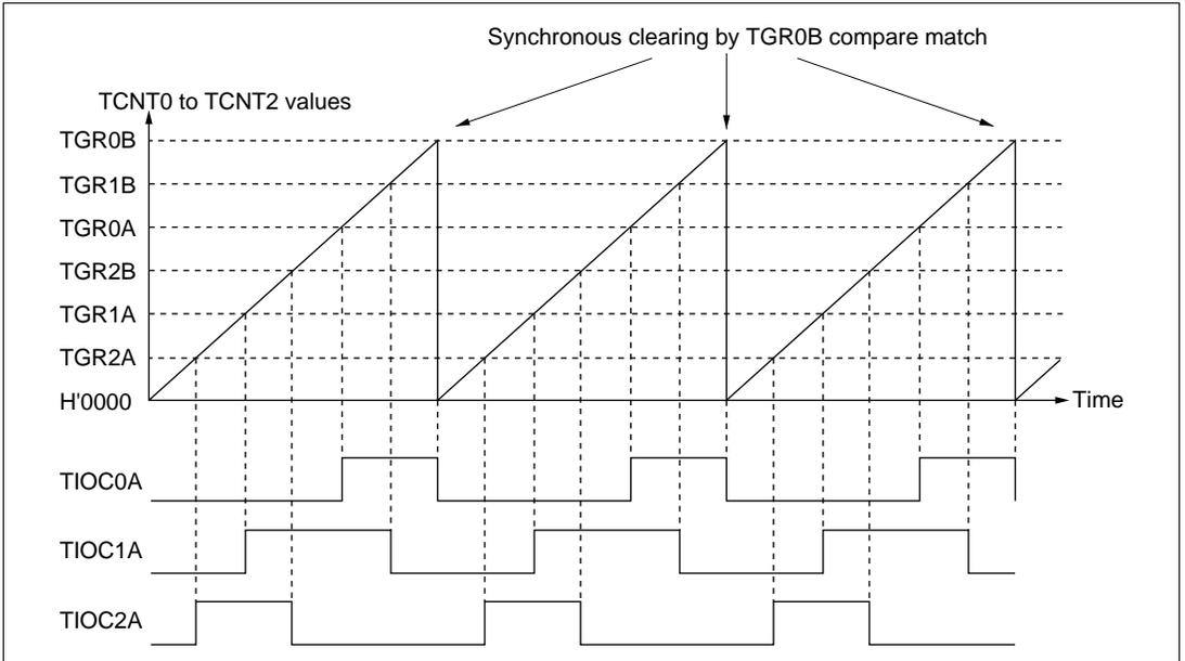
**Figure 9-15 Example of Synchronous Operation**
