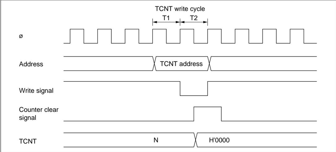
**Figure 9-45 Contention between TCNT Write and Clear Operations**
