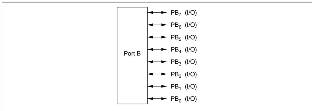
**Figure 8-13 Port B Pin Functions (Modes 3 and 7)**
