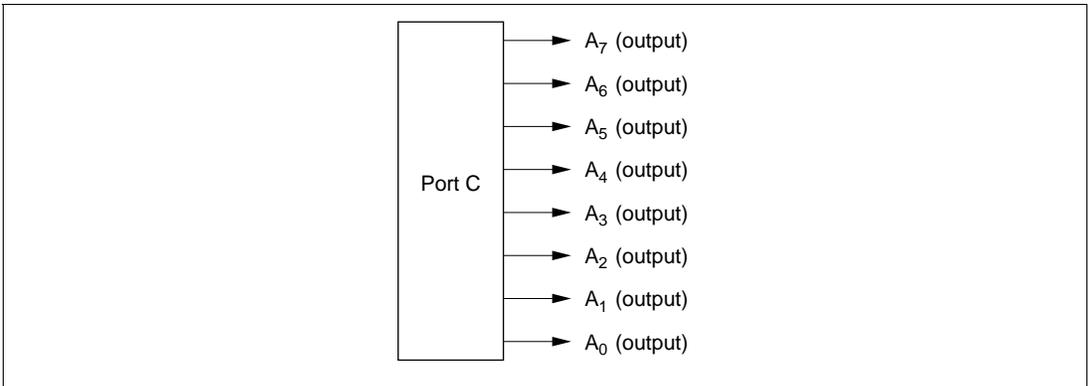
**Figure 8-15 Port C Pin Functions (Modes 1, 4, and 5)**
