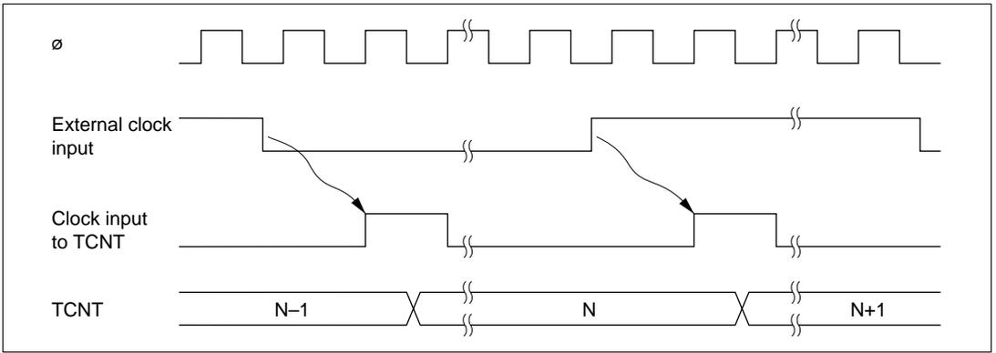
**Figure 10-3 Count Timing for External Clock Input**
