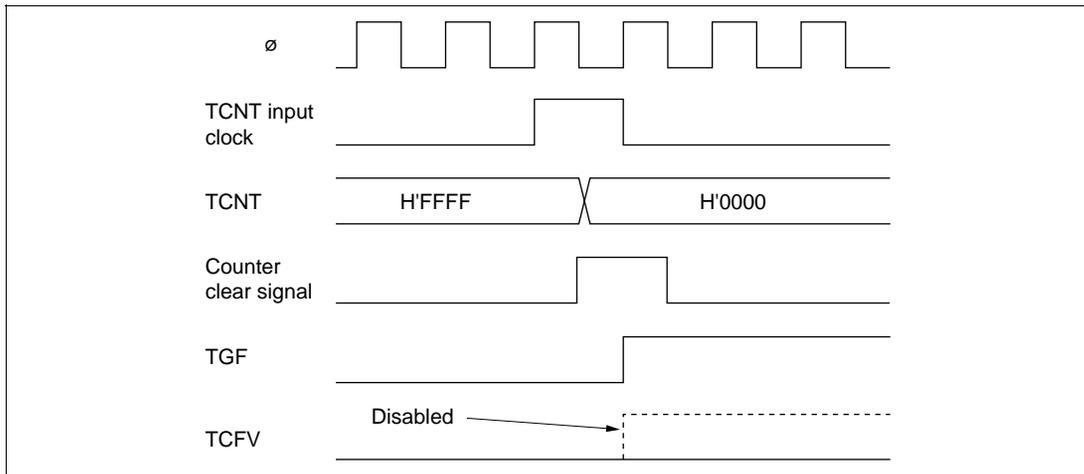
**Figure 9-52 Contention between Overflow and Counter Clearing**
