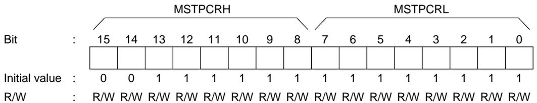
MSTPCR is a 16-bit readable/writable register that performs module stop mode control.
