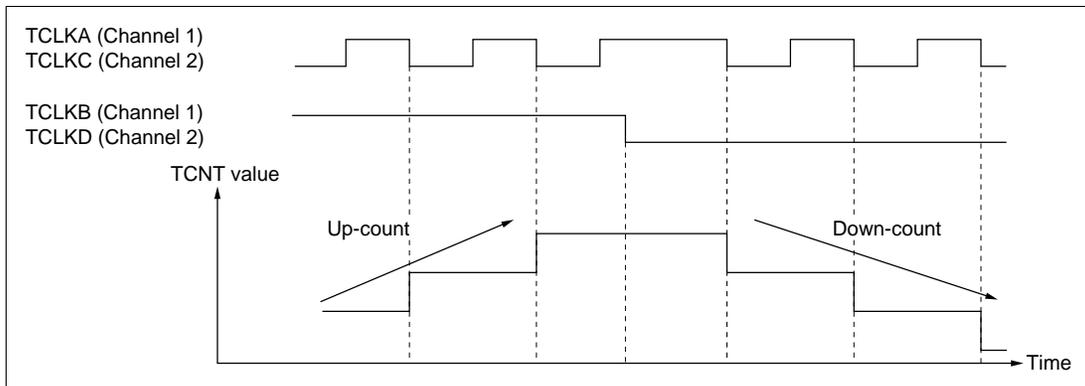
**Figure 9-27 Example of Phase Counting Mode 2 Operation**
