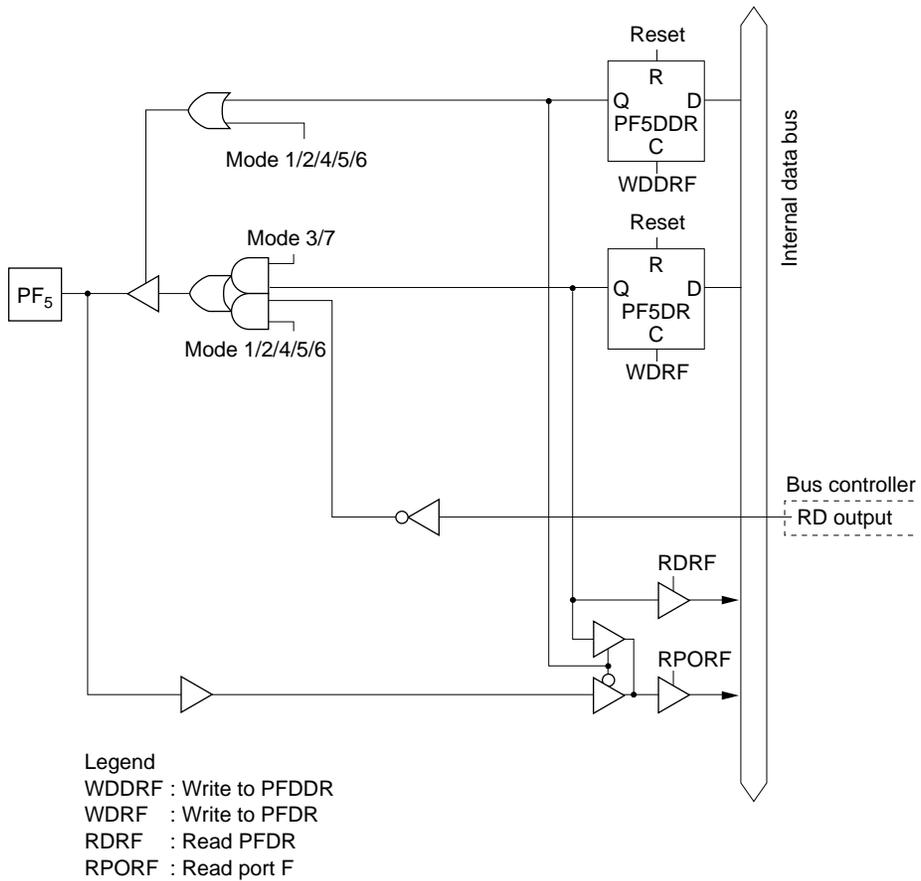
**Figure C-11 (f) Port F Block Diagram (Pin PF<sub>5</sub>)**
