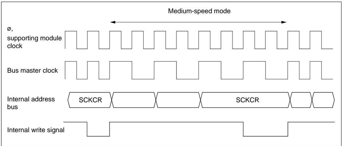
**Figure 18-1 Medium-Speed Mode Transition and Clearance Timing**
