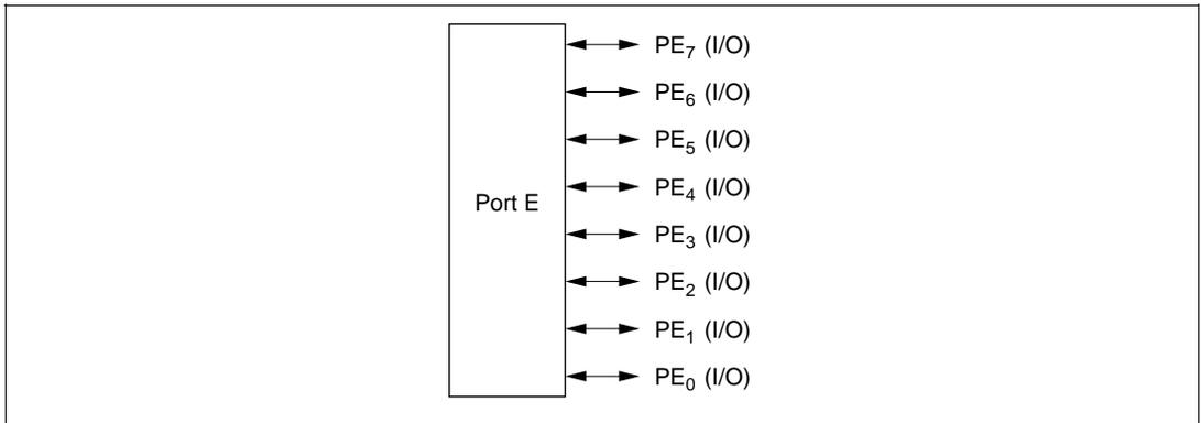
**Figure 8-23 Port E Pin Functions (Modes 3 and 7)**
