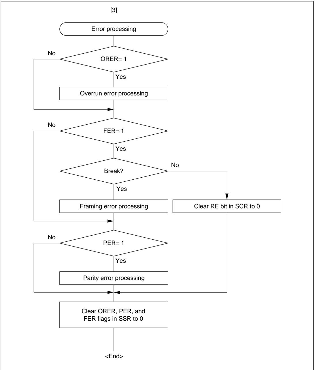
**Figure 12-7 Sample Serial Reception Data Flowchart (cont)**
