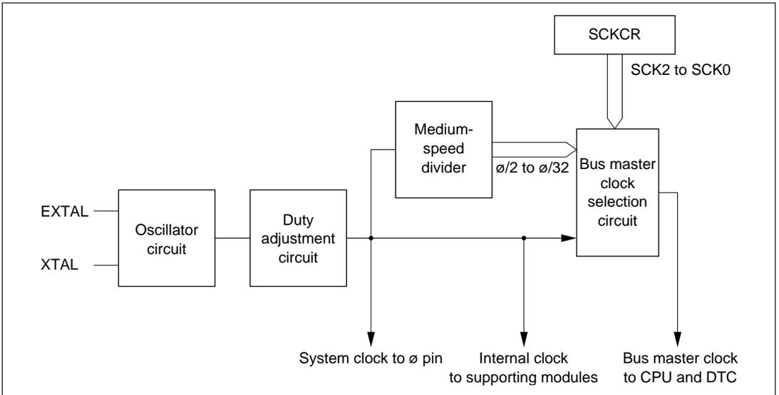
**Figure 17-1 Block Diagram of Clock Pulse Generator**
