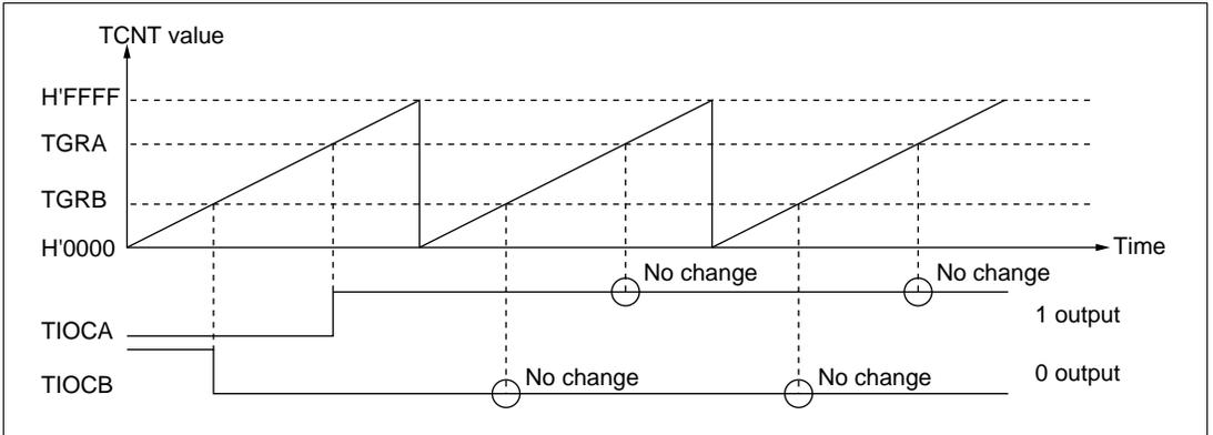
**Figure 9-10 Example of 0 Output/1 Output Operation**
