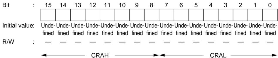
CRA is a 16-bit register that designates the number of times data is to be transferred by the DTC.
