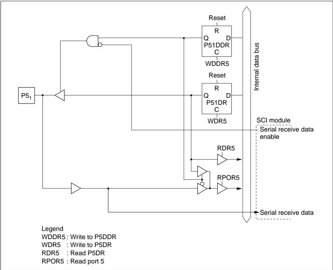
**Figure C-5 (b) Port 5 Block Diagram (Pin P5<sub>1</sub>)**
