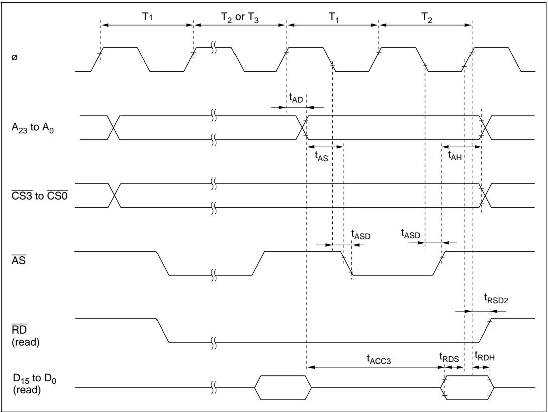
**Figure 19-11 Burst ROM Access Timing (Two-State Access)**
