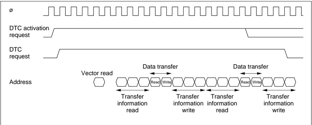
**Figure 7-12 DTC Operation Timing (Example of Chain Transfer)**
