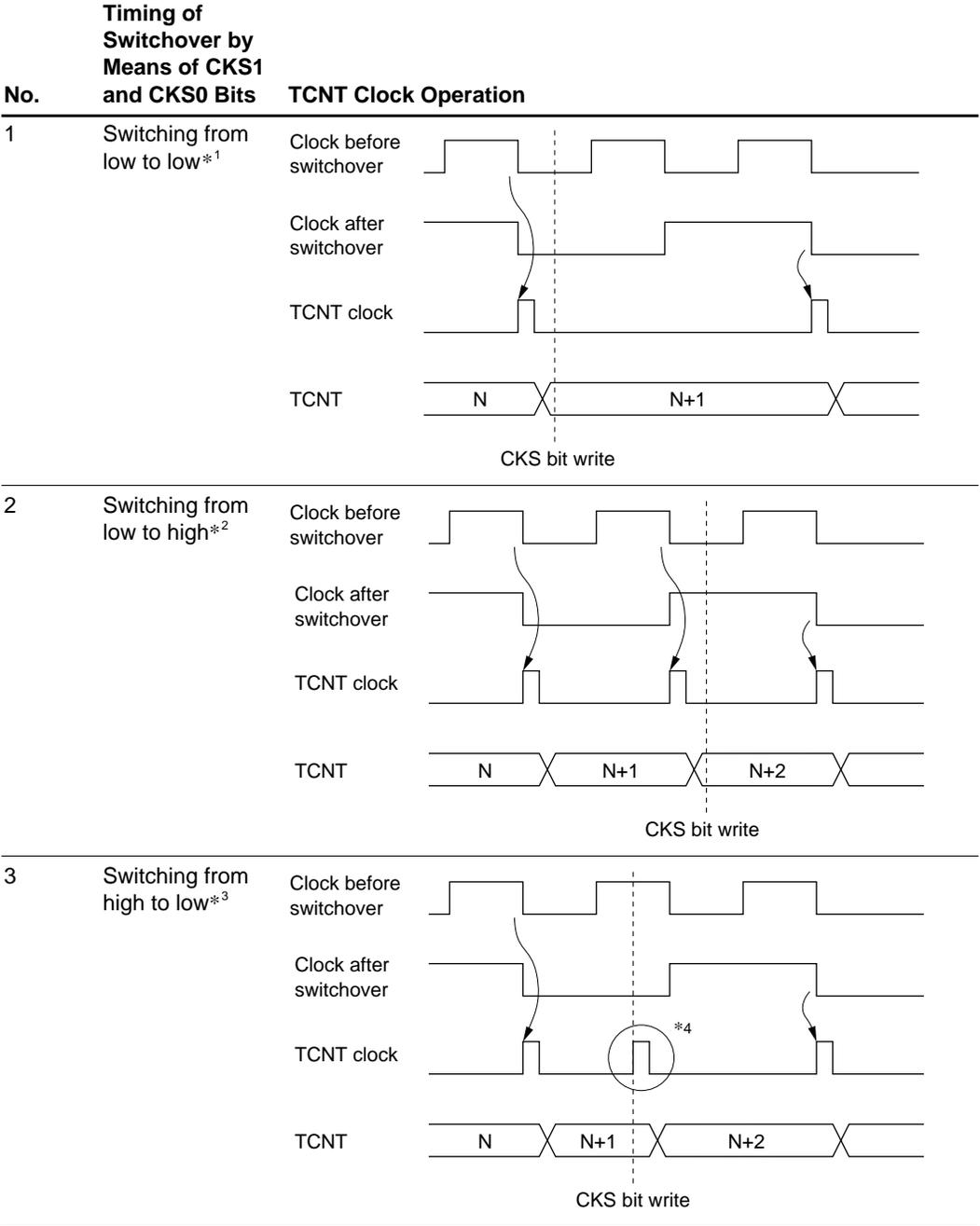
**Table 10-5 Switching of Internal Clock and TCNT Operation (cont)**
