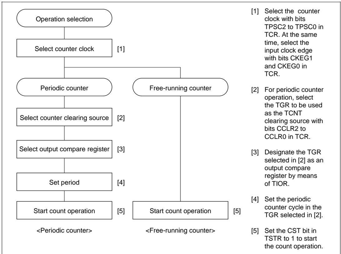
**Figure 9-6 Example of Counter Operation Setting Procedure**
