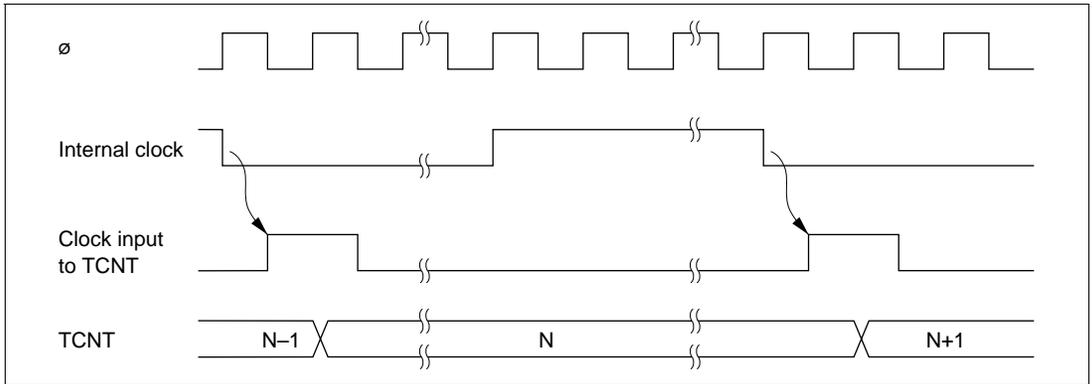
**Figure 10-2** Count Timing for Internal Clock Input
