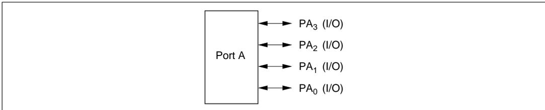
**Figure 8-7 Port A Pin Functions (Modes 1, 2, 3, and 7)**
