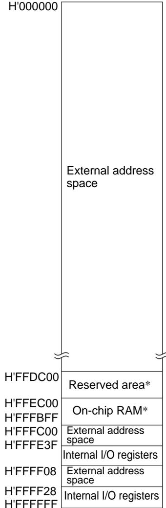
Note: \* External addresses can be accessed by clearing the RAME bit in SYSCR to 0.
