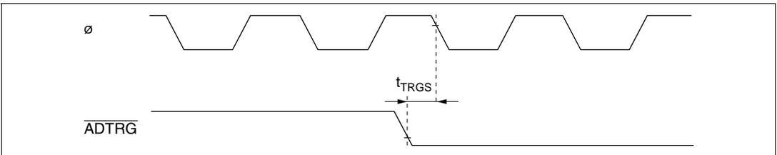
**Figure 19-24 A/D Converter External Trigger Input Timing**
