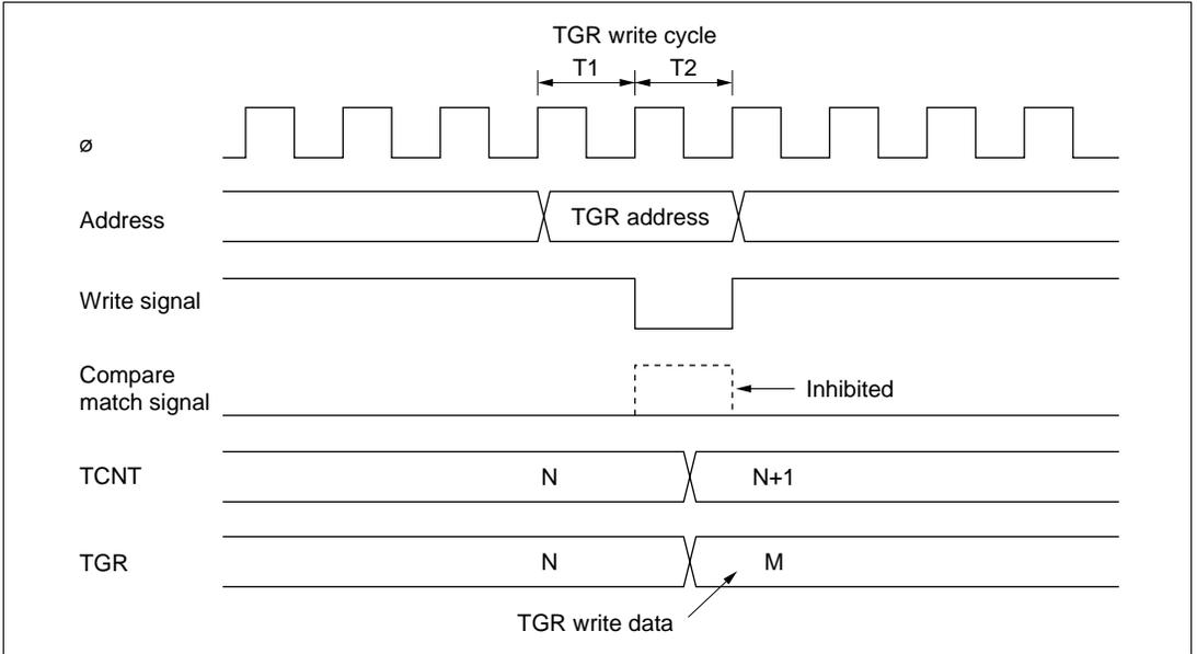
**Figure 9-47 Contention between TGR Write and Compare Match**
