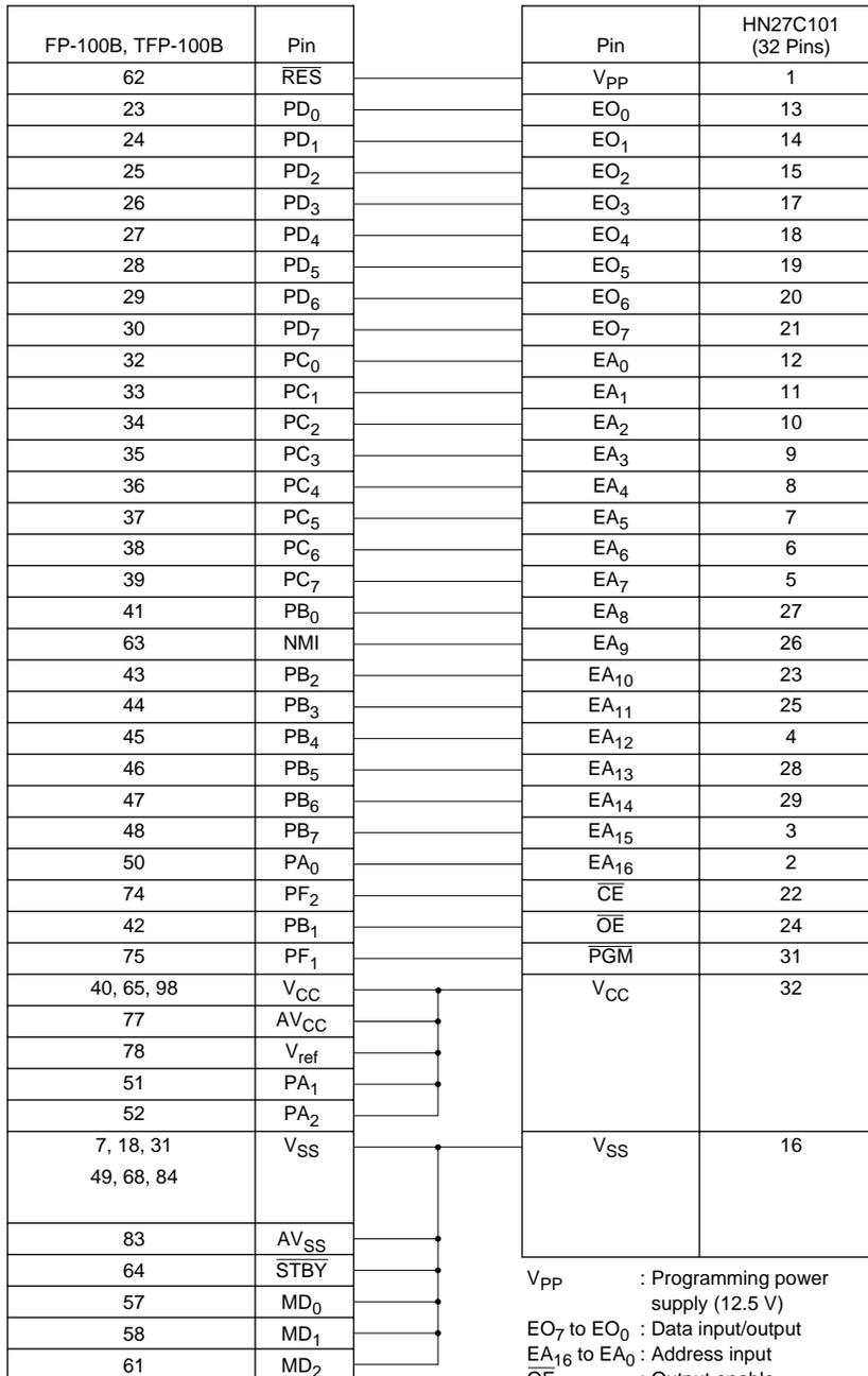
Note: Pins not shown in this figure should be left open.
