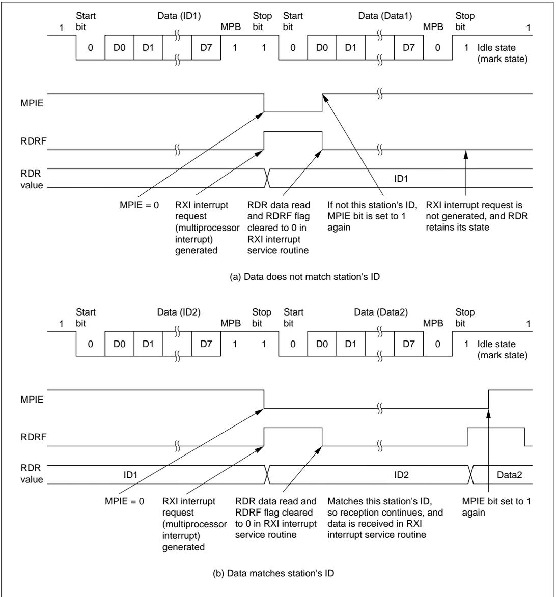
**Figure 12-13 Example of SCI Operation in Reception
