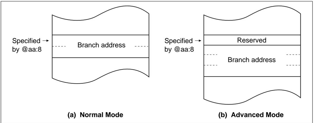
**Figure 2-13 Branch Address Specification in Memory Indirect Mode**
