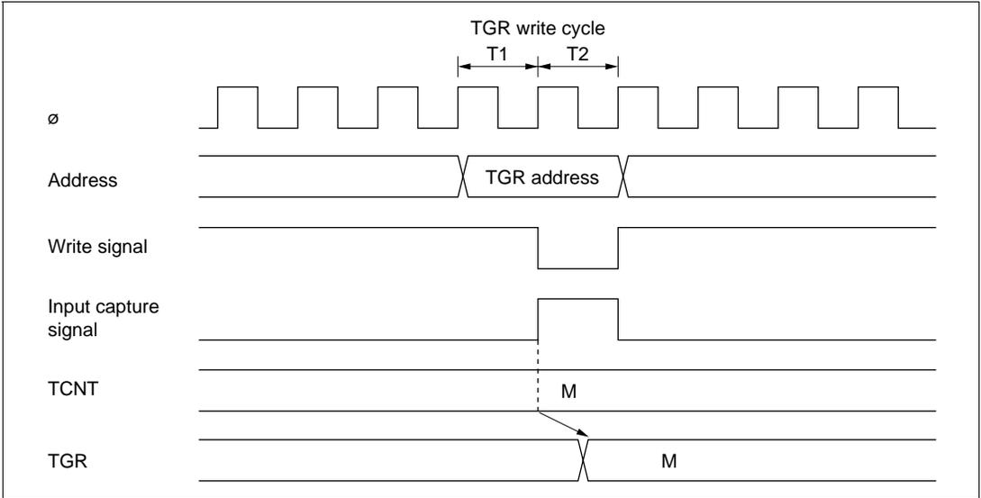
**Figure 9-50 Contention between TGR Write and Input Capture**
