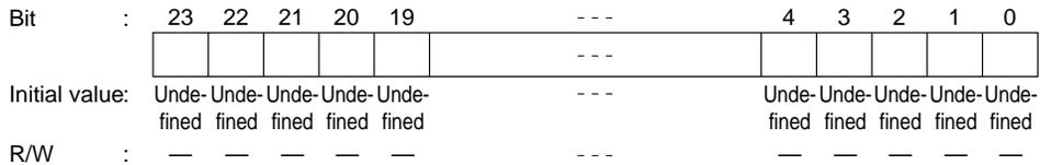
DAR is a 24-bit register that designates the destination address of data to be transferred by the DTC. For word-size transfer, specify an even destination address.
