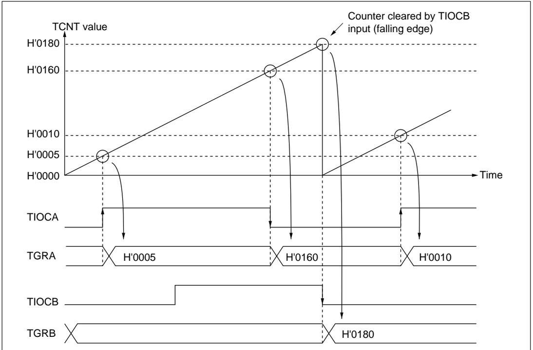
**Figure 9-13 Example of Input Capture Operation**
