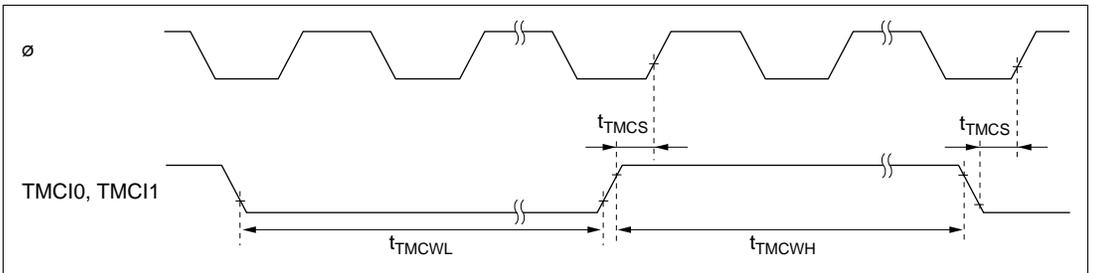
**Figure 19-19 8-Bit Timer Clock Input Timing**
