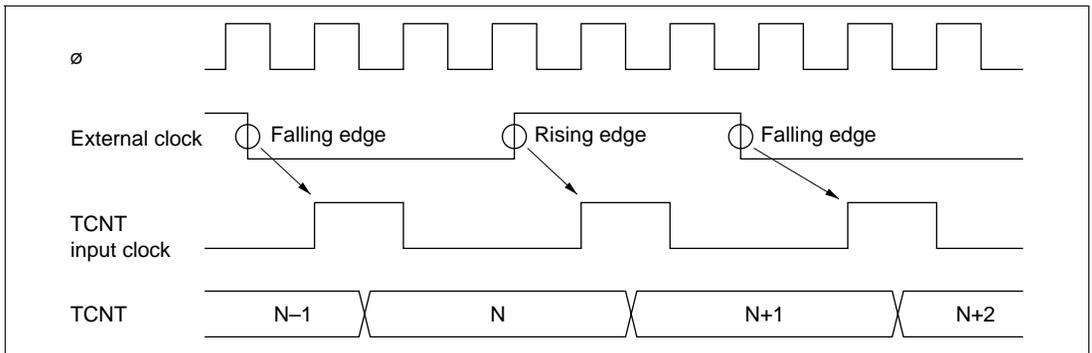
**Figure 9-31 Count Timing in External Clock Operation**
