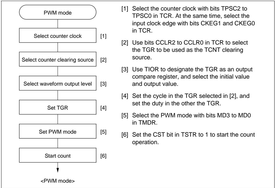
**Figure 9-21 Example of PWM Mode Setting Procedure**
