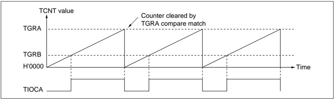
**Figure 9-22 Example of PWM Mode Operation (1)**
