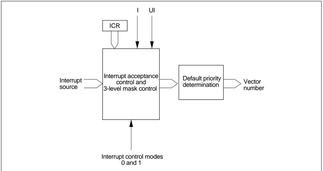
**Figure 5-4 Block Diagram of Interrupt Control Operation**
