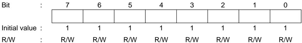
TDR is an 8-bit register that stores data for serial transmission.
