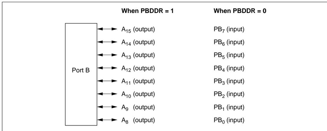
**Figure 8-12 Port B Pin Functions (Modes 2 and 6)**
