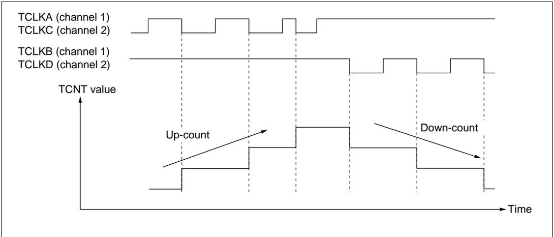
**Figure 9-28 Example of Phase Counting Mode 3 Operation**
