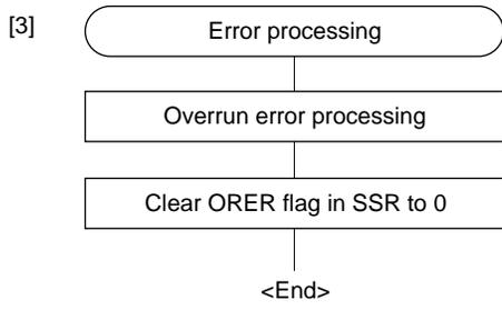
**Figure 12-18 Sample Serial Reception Flowchart**
