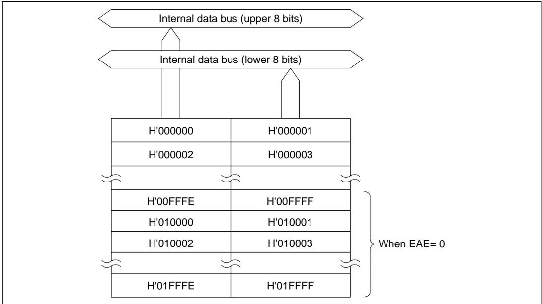
**Figure 16-1 Block Diagram of ROM (Example with H8S/2246 in Modes 6, 7)**
