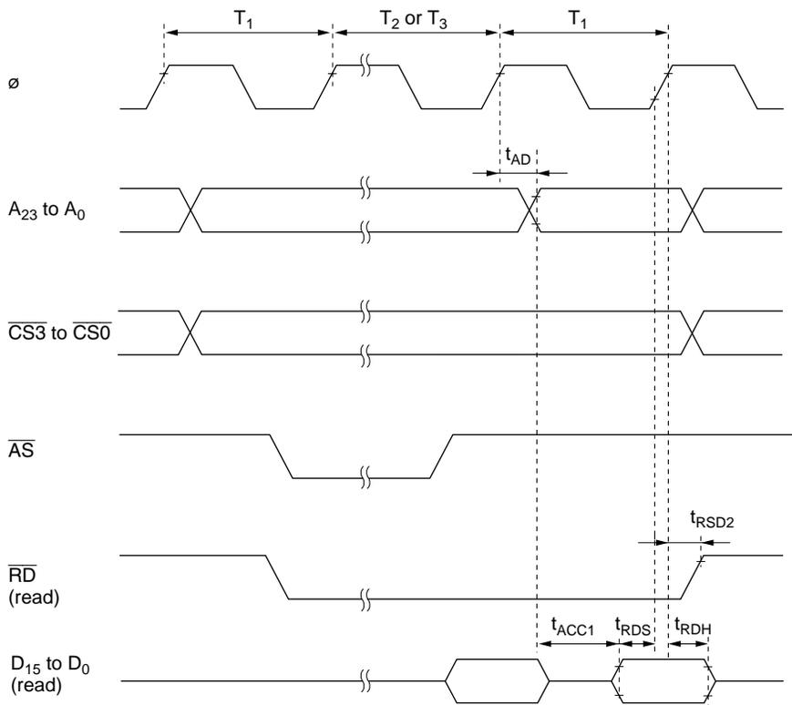
**Figure 19-12 Burst ROM Access Timing (One-State Access)**
