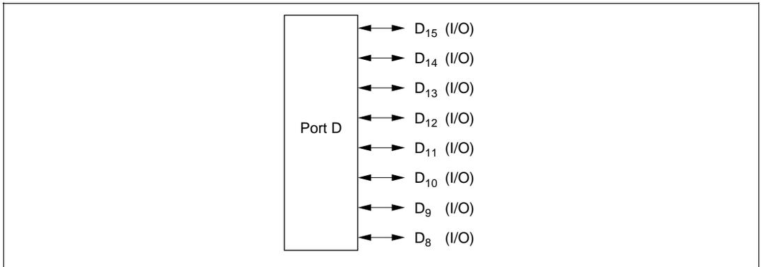
**Figure 8-19 Port D Pin Functions (Modes 1, 2, 4, 5, and 6)**
