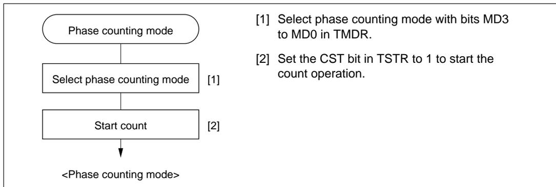
**Figure 9-25 Example of Phase Counting Mode Setting Procedure**
