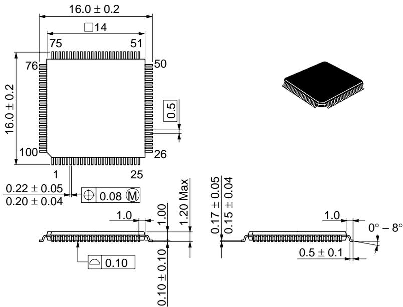
Dimension including the plating thickness
