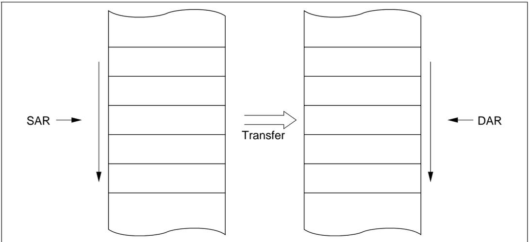
**Figure 7-6 Memory Mapping in Normal Mode**
