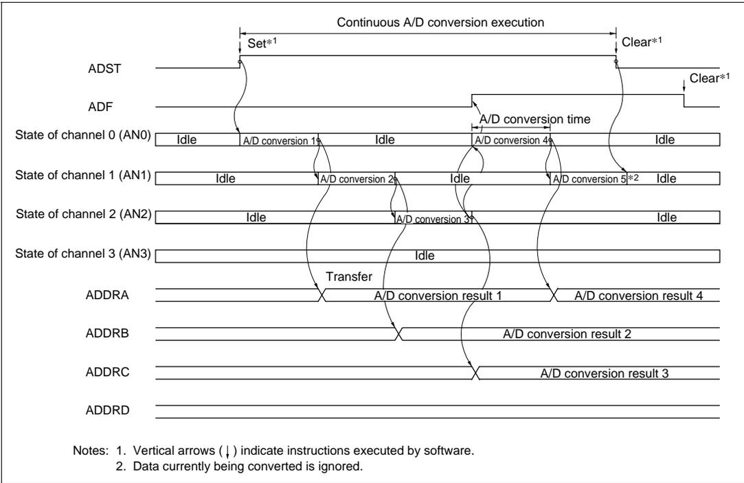
**Figure 14-4 Example of A/D Converter Operation
