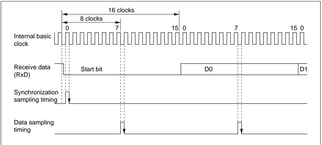
**Figure 12-21 Receive Data Sampling Timing in Asynchronous Mode**
