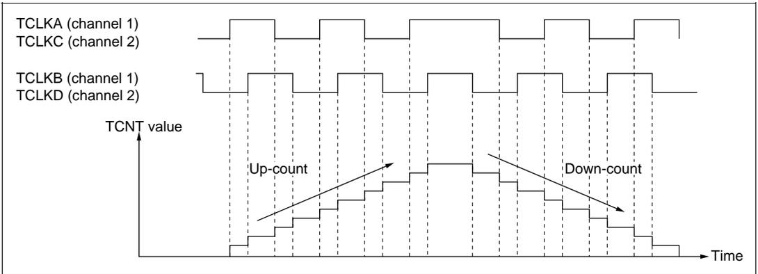
**Figure 9-26 Example of Phase Counting Mode 1 Operation**
