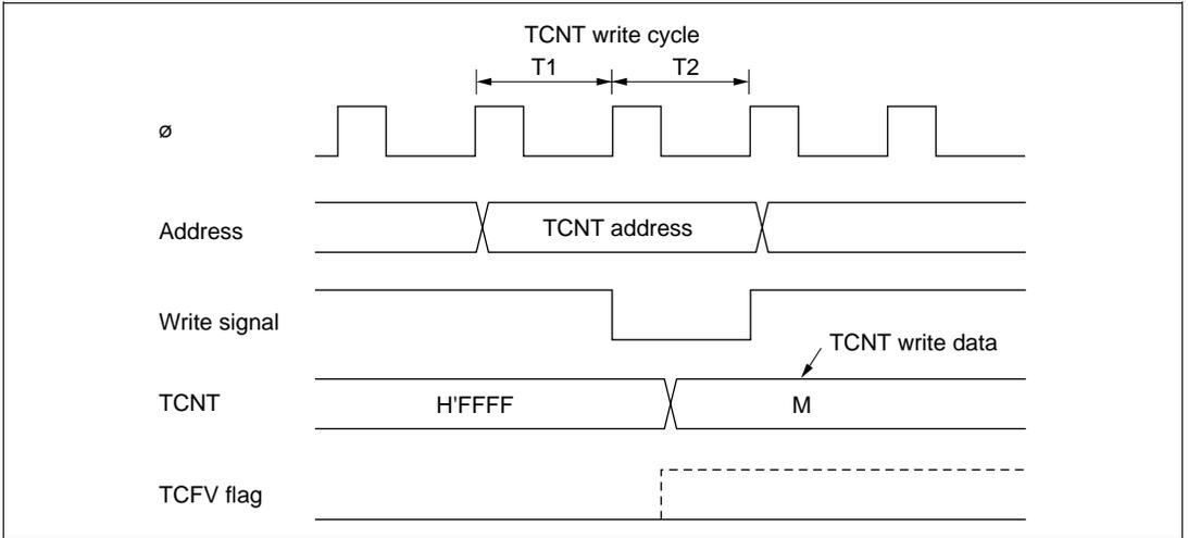
**Figure 9-53 Contention between TCNT Write and Overflow**
