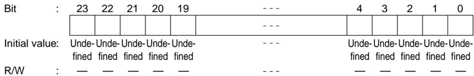
SAR is a 24-bit register that designates the source address of data to be transferred by the DTC. For word-size transfer, specify an even source address.
