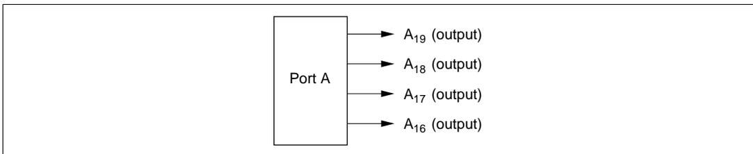
**Figure 8-8 Port A Pin Functions (Modes 4 and 5)**
