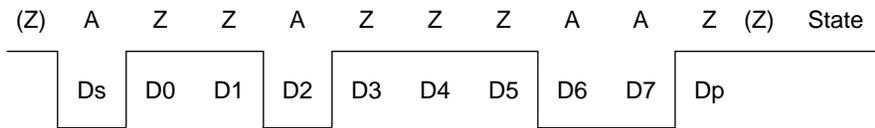
With the direct convention type, the logic 1 level corresponds to state Z and the logic 0 level to state A, and transfer is performed in LSB-first order. The start character data above is H'3B.
