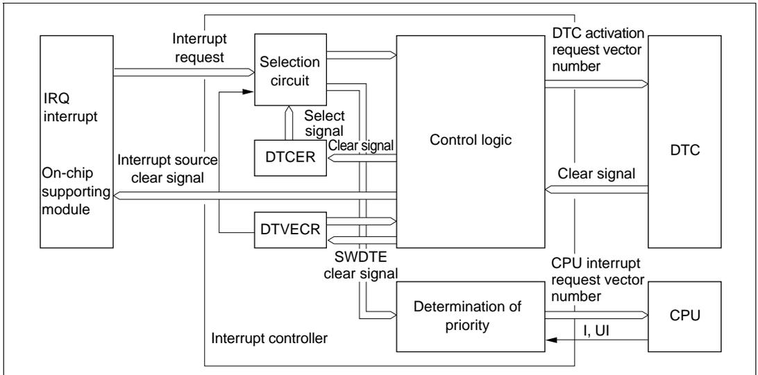
**Figure 5-10 Interrupt Control for DTC**
