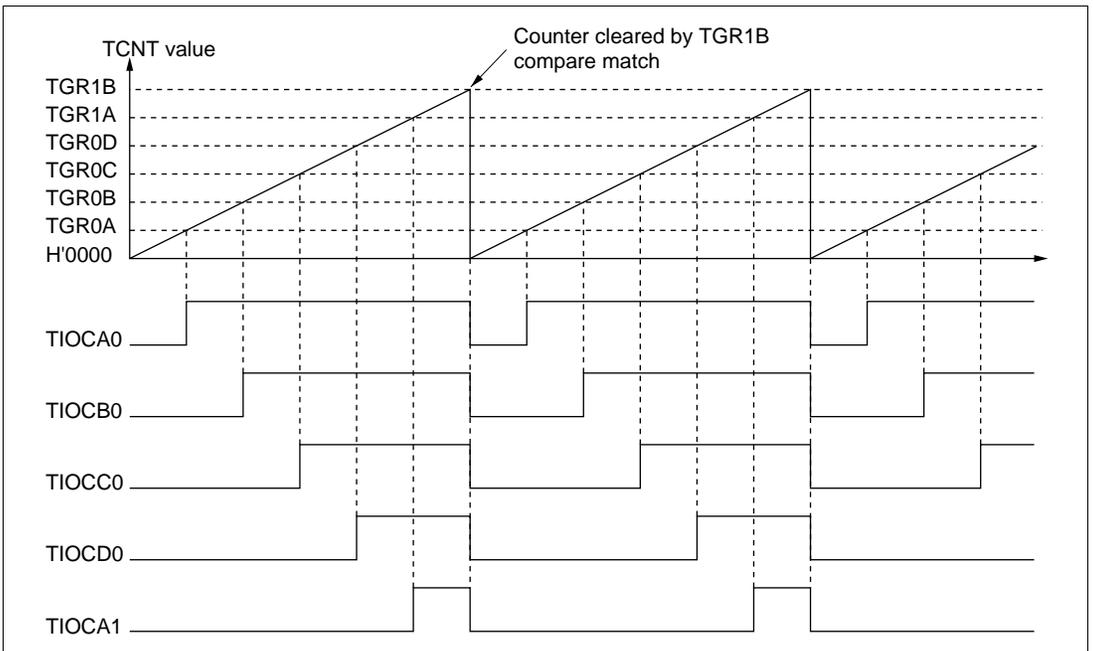
**Figure 9-23 Example of PWM Mode Operation (2)**
