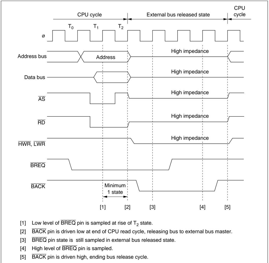
**Figure 6-19 Bus-Released State Transition Timing**
