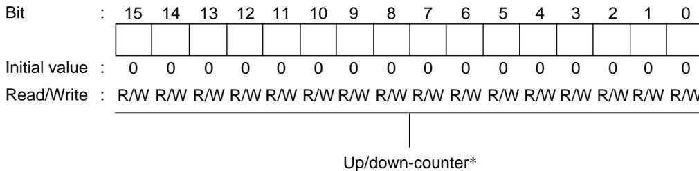
Note: \* This timer counter can be used as an up/down-counter only in phase counting mode or when performing overflow/underflow counting on another channel. In other cases it functions as an up-counter.
