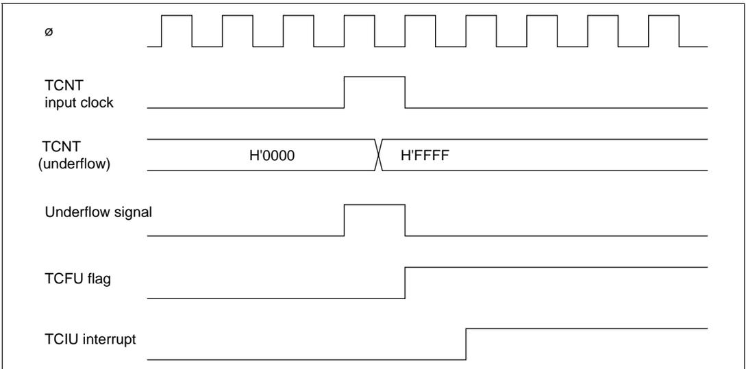
**Figure 9-41 TCIU Interrupt Setting Timing**
